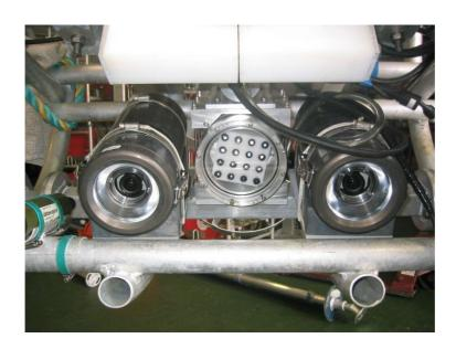
Figure 13.5.2.1 Laser projection system mounted between stereo cameras
