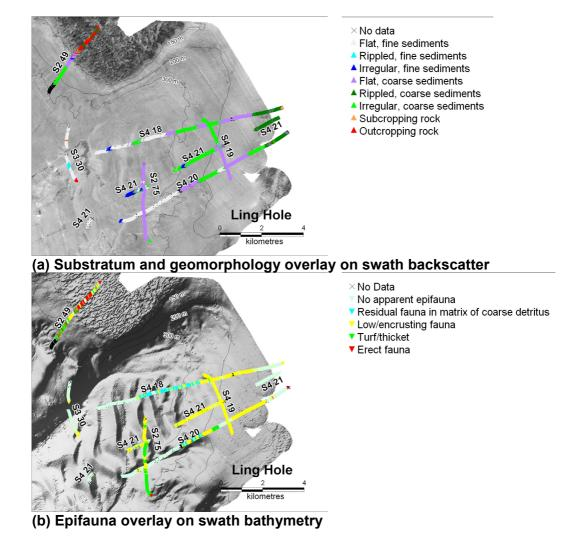
Figure 7.1.2.5 Ling Hole: map of survey site showing attributes overlaid on seabed (a) backscatter and (b) bathymetry. Each attribute is scored at 1-second intervals and mapped thematically: (a) substratum and geomorphology; (b) epifauna.
