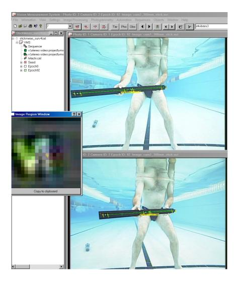
Figure 13.5.1.2 Paired images from the stereo cameras from the in-water verification of measurement accuracy following calibration of the cameras. Measurements between reflective targets on an aluminium rod were made at various rotations, distances and angles.
