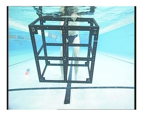
Figure 13.5.1.1 The in-pool calibration of the stereo cameras using a cube frame with reflective circular targets and 'coded targets' for automated recognition by the calibration software. A flashing red light enabled synchronization of the image pairs during analysis.
