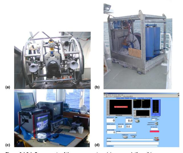
Figure 6.1.2.1 Components of the camera system: (a) camera platform (b) custom-built electric-hydraulic winch and (c &d) the bridge control set-up with monitors having real-time video feed, joystick remote control of the winch to control depth off sea-floor and a computer with (d) LabView console showing real-time position and telemetry read-outs
