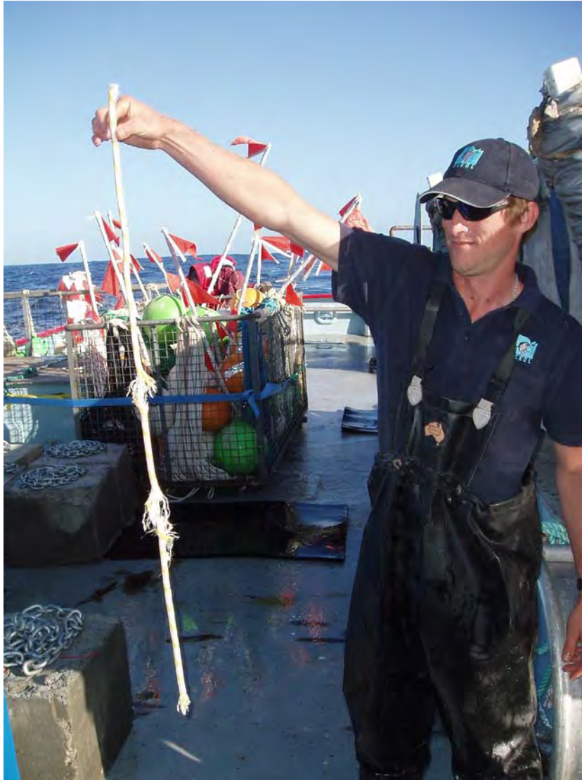
Figure 3. The 14mm double braid mooring rope severed by a shark resulting in the mooring drifting free.
