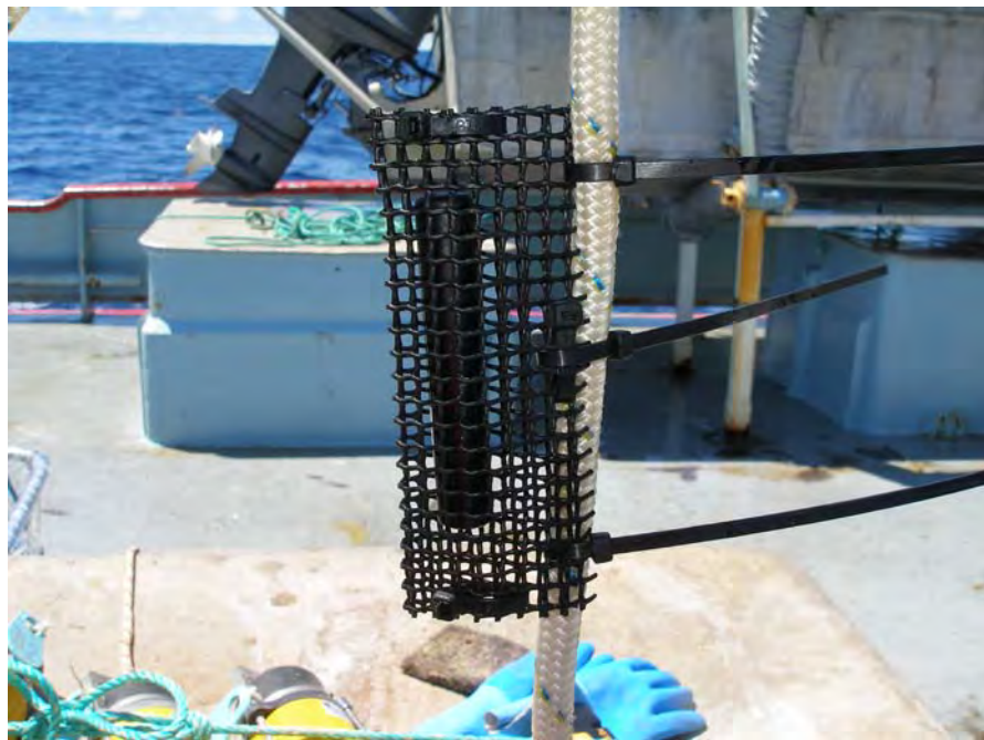
Figure 6. The range-test tag enclosed in plastic mesh and attached to the mooring rope using cable ties.
