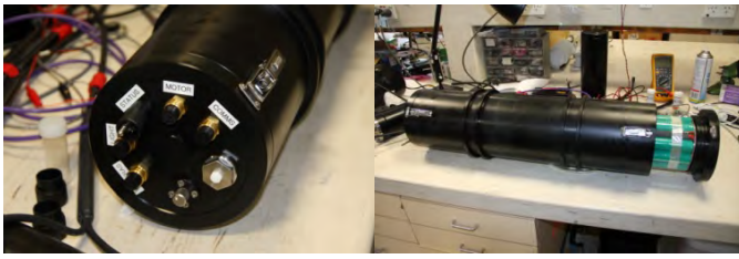
Figure 7. (L) Electronics housing connectors and interface. (R) Complete electronics housing with battery pack showing.
