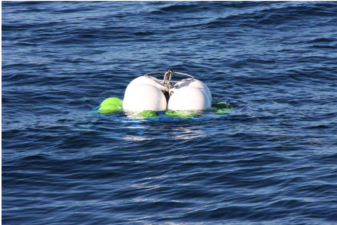
Figure 3. The DeepBRUVS at the surface following ascent from the bottom with release of the weights.
