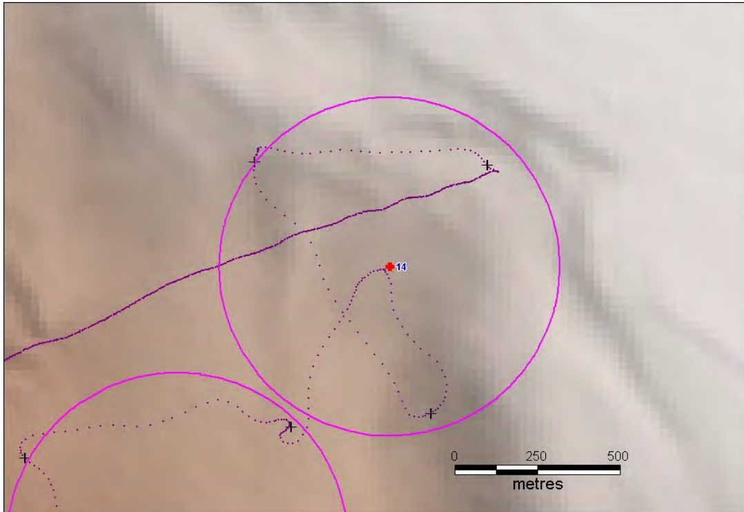
Figure 4. The vessel track (magenta dots) and locations for CART ranging (black crosses) as completed for each new mooring deployment. The red cross is the target location for deployment and the pink circle shows the ~500 m range of detection for the VR2. The ranging of the CARTS enables accurate determination of the location of the mooring on the sea floor with post processing.
