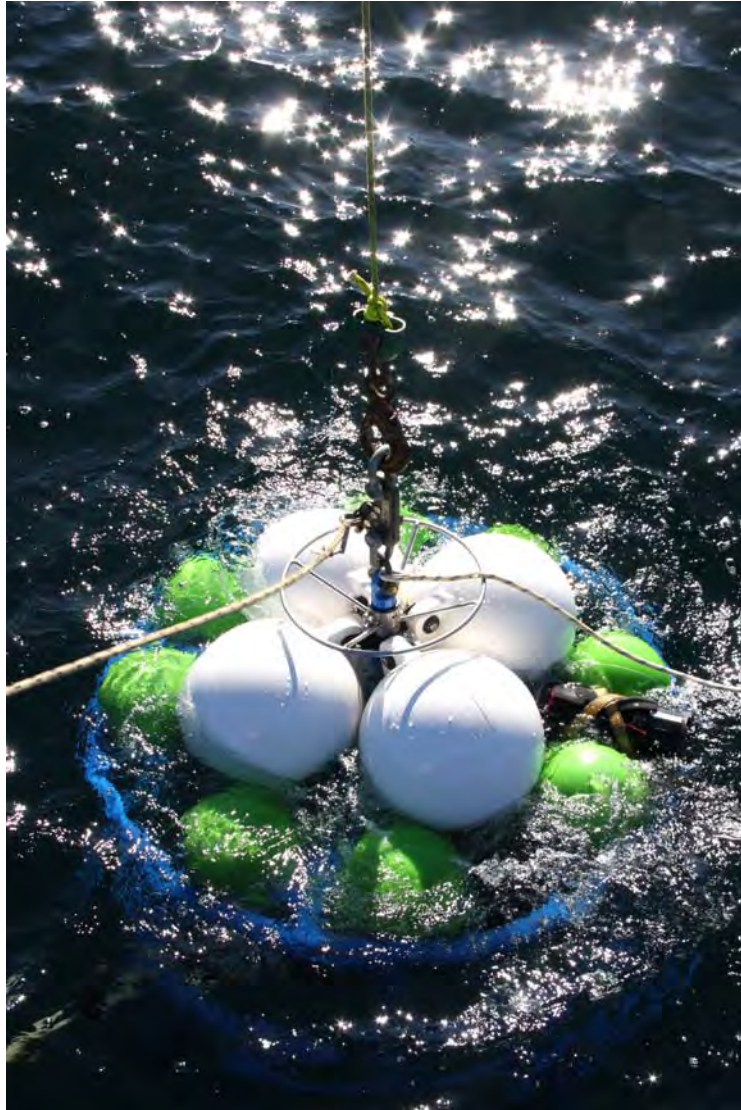
Figure 5. The DeepBRUVS in the water at the side of the vessel just prior to detaching via the 'Sea Catch' release
