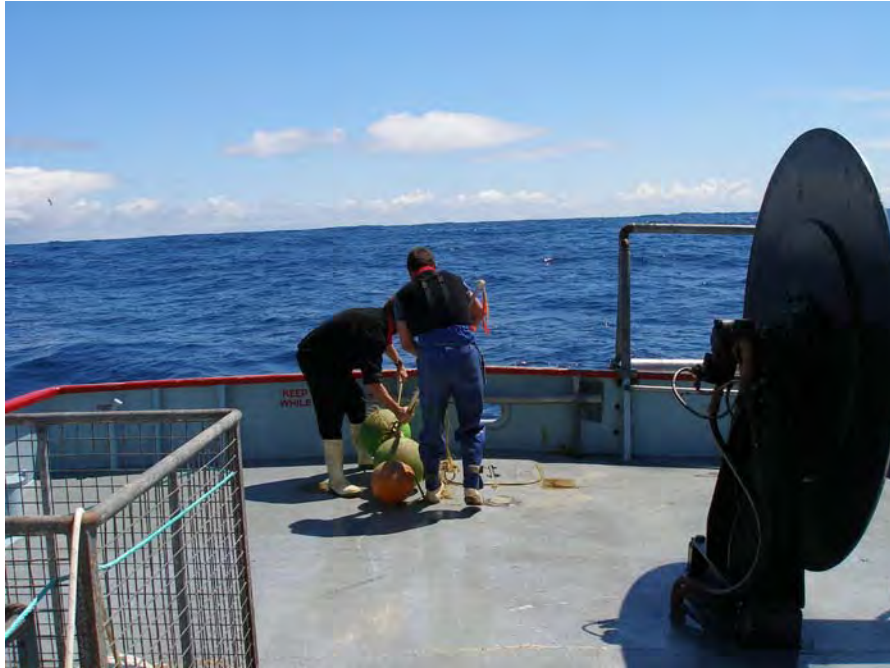
Figure 5. The surface floats are brought on board following release and ascent from 100 meters off bottom.
