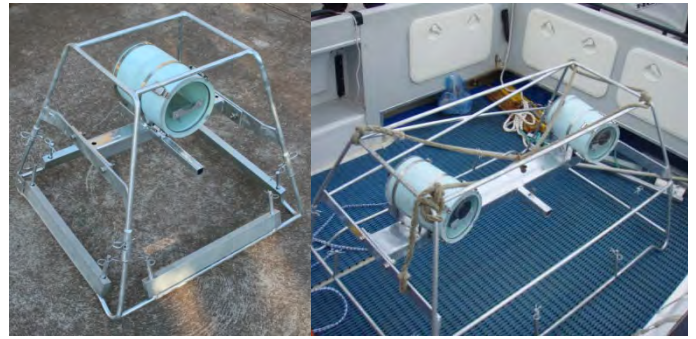
Figure 1. Conventional 2D(L) and 3D(R) BRUVS systems.
