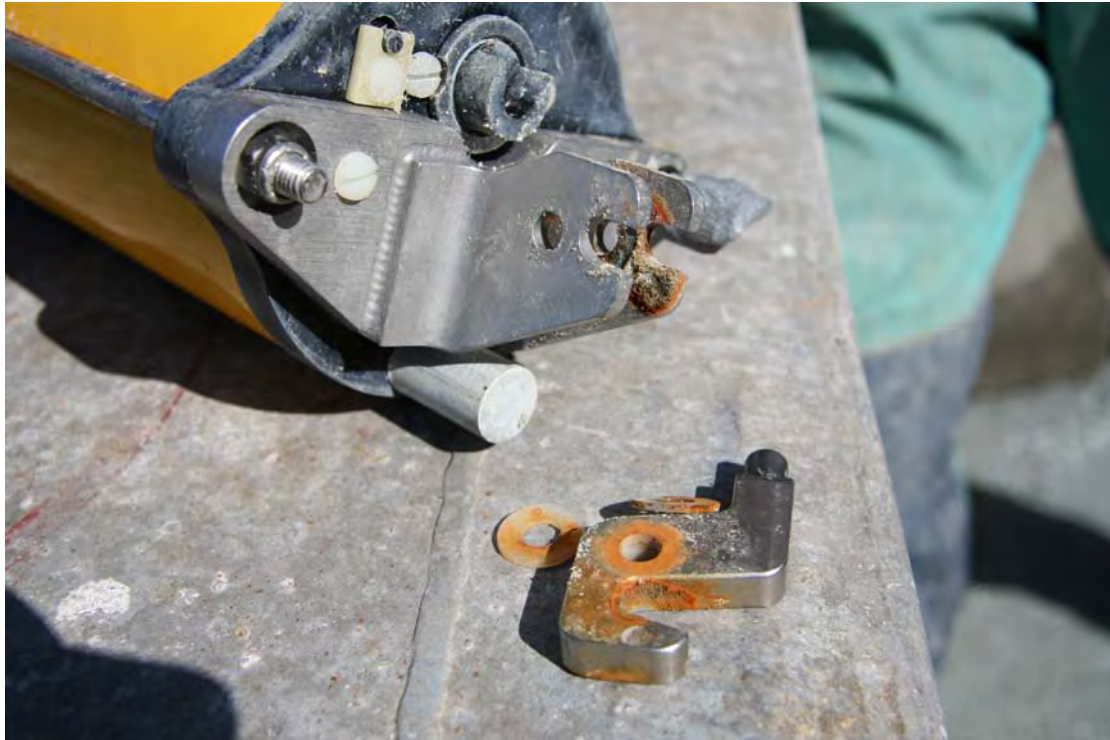
Figure 2. One of the CART units showing the corrosion on the release mechanism that may have been contributing to the release failure of some of the other moorings.
