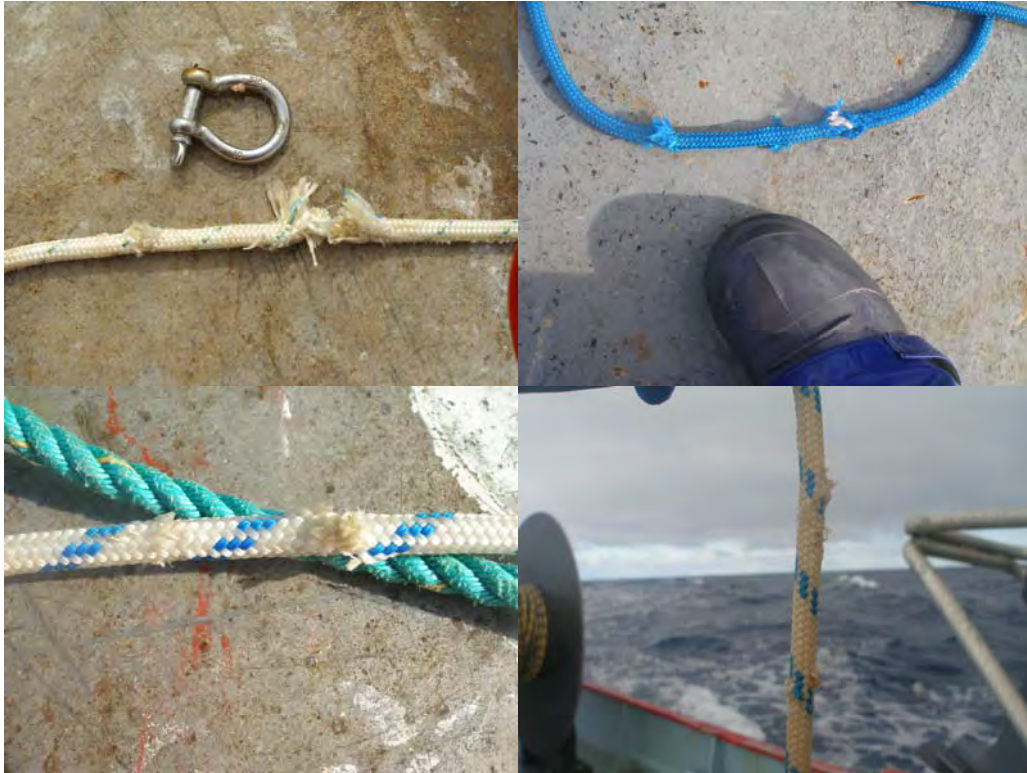
Figure 7. Images showing damage, at varying levels of severity, to the mooring lines. It is most likely the damage is from shark and or fish i.e. leather jackets biting the rope. Not all ropes were damaged, probably only 20% had damage. In many cases the overall strength of the rope wasn't compromised significantly, whereas in one case we were probably fortunate to get the mooring back at all as it was attached by only by the inner core
