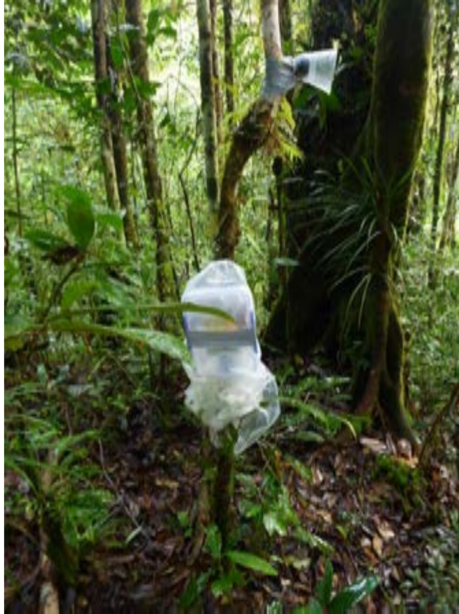
Figure 5. Method of deployment of an AnaBat SD1 unit for passive acoustic recording of insectivorous bats. The microphone is located within the plastic cone which protects it from rain.
