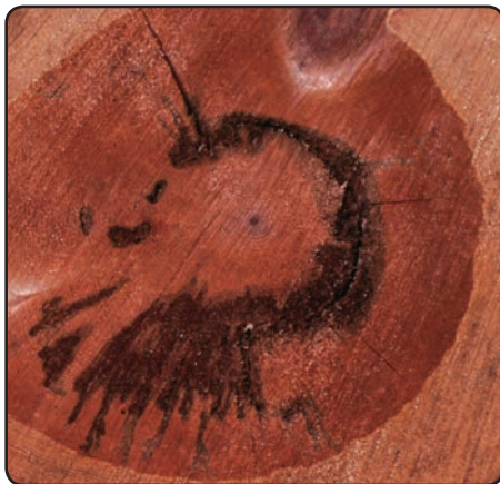
Figure 200. Red rot decay affects the heartwood and is typically associated with old growth ponderosa pine.
