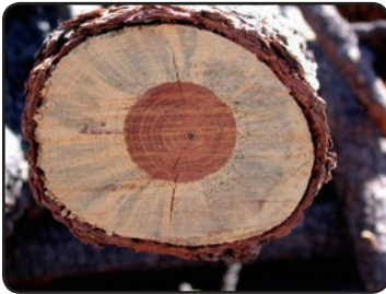
Figure 89. Blue stain fungi introduced during bark beetle attacks on conifers occurs in the sapwood.
