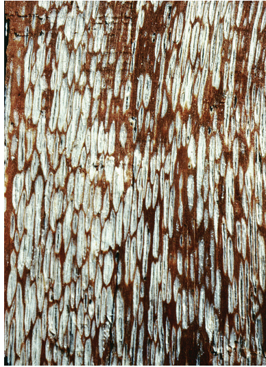
Figure 4. Typical white pocket rot of Porodaedalea ( Phellinus ) pini with white pockets bordered by reddish, relatively undecayed wood. Photo: Jim Worrall, USDA Forest Service.
