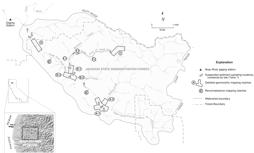
Figure 1 —Drainage map of the South Fork Noyo River watershed showing detailed geomorphic mapping locations, reconnaissance mapping reaches, suspended sediment sampling locations, cross section locations, watershed boundary, and property boundary of Jackson State Demonstration Forest.
