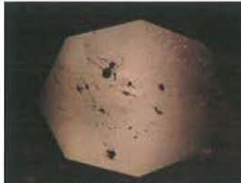
Figure 49: RGC006 as in RGC007, RGC 010 and RGC011this NTSR image of the table facet also reveals a virtual jigsaw puzzle of glass and ruby – islands of ruby in a glass matrix
