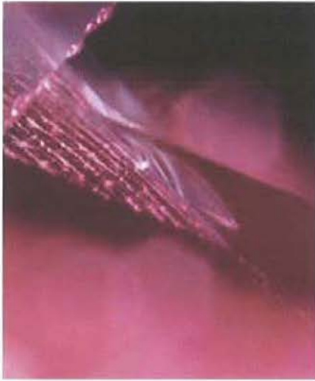
Figure 6: Another feature of the spinels heated at relatively lower temperatures was the occurrence of very transparent, subtle stress fractures extending from the constituents of healed fissures. (Photomicrograph: Christopher P. Smith, 75x)
