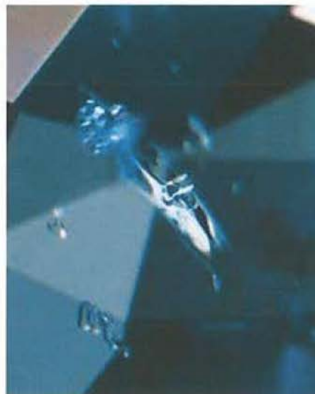
Figure 7: Mineral inclusions of the spinels heated at relatively lower temperatures also revealed evidence of this treatment. Shown here are inclusions of apatite with thermally induced stress fractures. (Photomicrograph: Christopher P. Smith, 65x)
