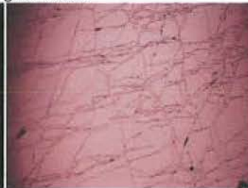
Figure 44: RGC010 (magnified from Figure 43) as in RGC007 this NTSR image of the table facet also reveals a virtual jigsaw puzzle of glass and ruby – islands of ruby in a glass matrix
