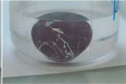
Figure 65: RGC015 seen here immersed in hydrofluoric acid. The white substance is residue from disintegration of the glass by the acid. The disintegration process begins as soon as the stone is placed in the acid. This image is taken within 30 minutes of immersion.
