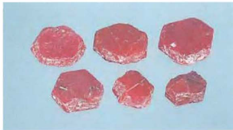
Figure 4. The starting material for this ruby treatment is very low quality and until now was only useful as mineral specimens. The crystals shown here range from 7.28 to 22.08 ct. Photo by Maha Calderon.
