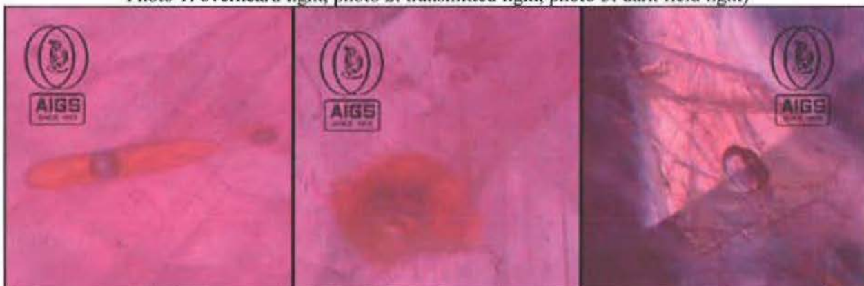
(Other cavities filled with orange lead rich glass in "Bangkok repaired" rubies. Photos: Transmitted light)
