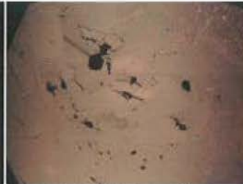
Figure 50: RGC006 (magnified from Figure 49) as in RGC007, RGC 010 and RGC011this NTSR image of the table facet also reveals a virtual jigsaw puzzle of glass and ruby – islands of ruby in a glass matrix
