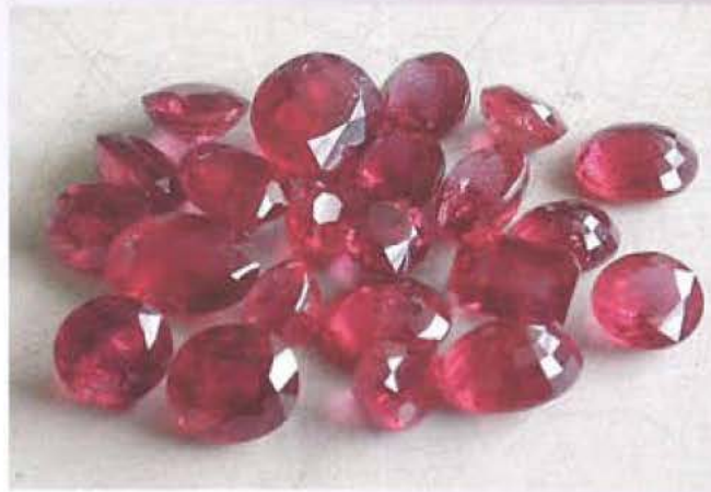
Rubies found with lead rich foreign substance filling in fissures and cavities at the AIGS laboratory.
