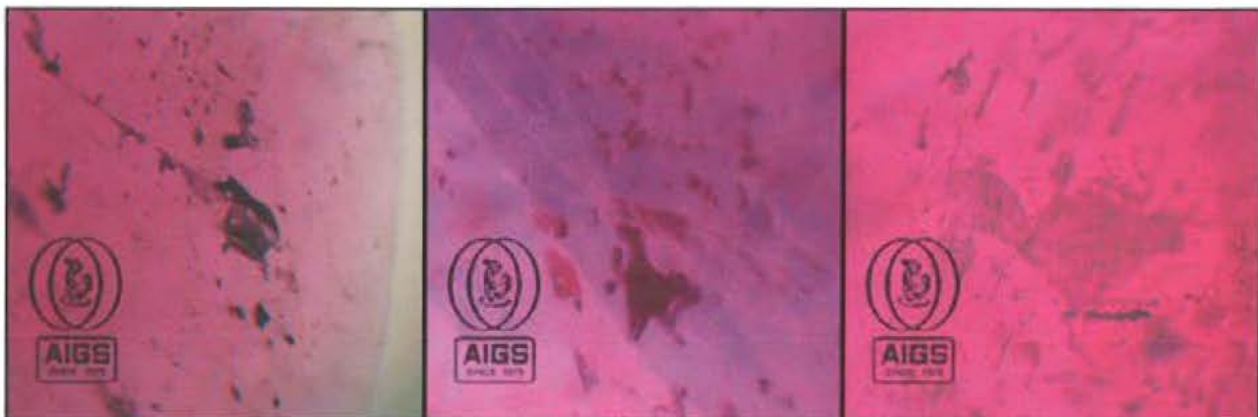
("Platelets" found in Chantaburi rubies: They are transparent or act as mirrors depending the light orientation.)
