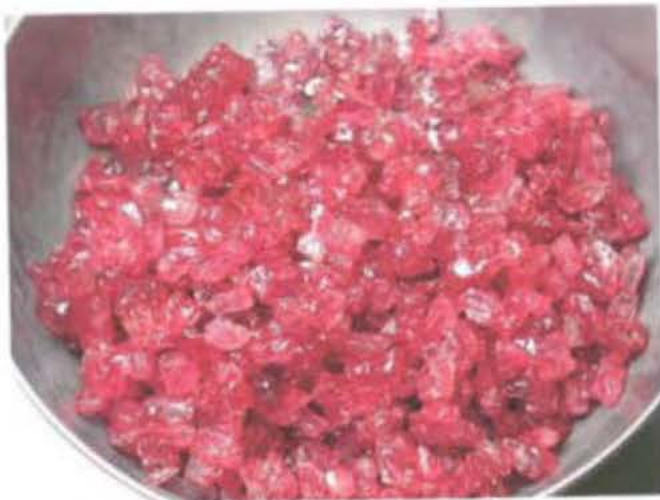
After heating, the chemicals form a glass coating as seen in this dish of ruby rough.
