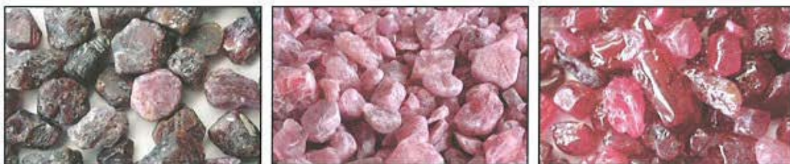
Figure 3: Left: Rough ruby material from Andilamena as found at the mines. Center: The same Andilamena material after cleaning fissures with acid and a preliminary heat treatment step without additives in order to clean the fissures to enable the final lead glass treatment. Right: The same Andilamena ruby material after the final heat treatment with lead glass. Photos: V. Pardieu / AIGS, 2005
