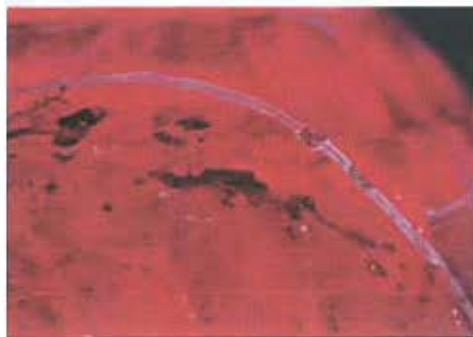
Figure 23. The large fracture in this lead glass-filled ruby is hard to see (left), except for the straight edges on the two flattened gas bubbles in the top center. After immersion in a standard pickling solution for 20 minutes (right), etching of the filler made the edges of the fracture clearly visible. Photomicrographs by S. F. McClure; magnified 30x.
