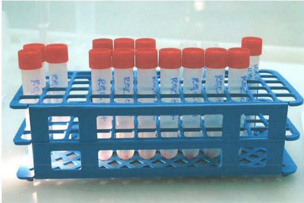
Figure 2: A rack holding individual plastic tubes that held the specimens that underwent acid disintegration. The stones were placed into the tubes and then covered with hydrofluoric acid 4 sealed and left to “soak” for from two to ten days.
