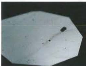
Figure 52: RGC002 showing a wide tract of glass crossing the table facet in NTSF, two bubbles are seen cut through at the surface
