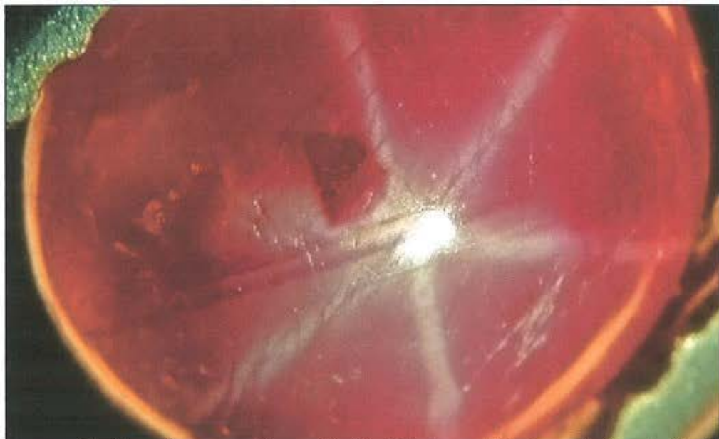
Figure 11: In stones like this one the presence of large cavities filled with glass, containing large spherical gas bubbles (left of the stone) can help to identify the presence of glass filling. Nevertheless the luster difference is not obvious and in such milky stones the examination of the fissures is difficult. Photo: V. Pardieu.
