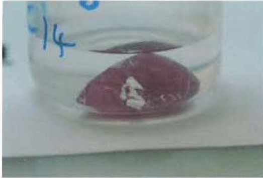
Figure 64: RGC014 seen here immersed in hydrofluoric acid. The white substance is residue from disintegration of the glass by the acid. The disintegration process begins as soon as the stone is placed in the acid. This image is taken within 30 minutes of immersion.
