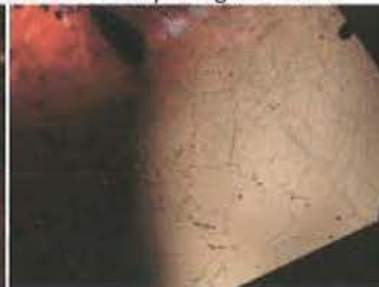
Figure 47: RGC011 (magnified from Figure 46) as in RGC007 and RGC 010 this NTSR image of the table facet also reveals a virtual jigsaw puzzle of glass and ruby – islands of ruby in a glass matrix
