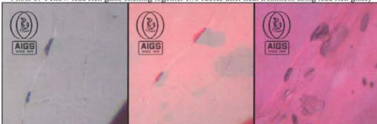
(A wide fissure filled with lead glass from a "Bangkok repaired" ruby present a noticeable orange color: Left to right: overhead, transmitted and dark field illumination)
