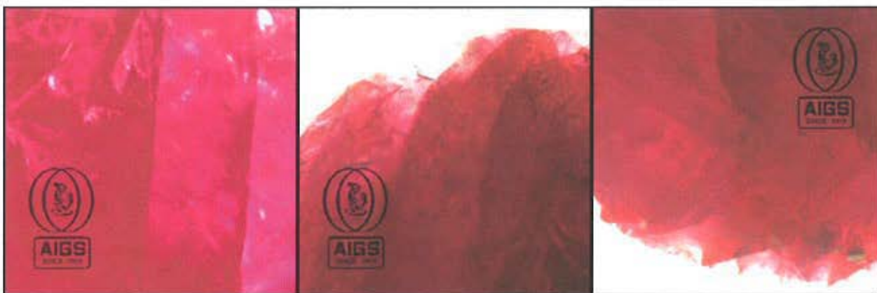
(Typical dyed rubies presenting strong red colored fissures and a very lightly colored body color)
