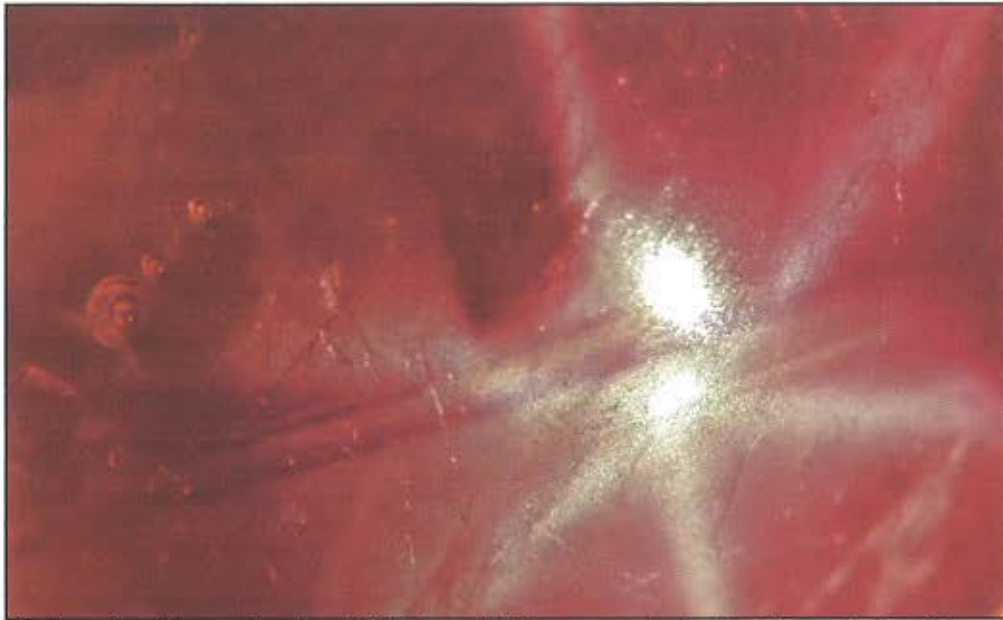
Figure 12: A closer view of the previous stone. Whilst the gas bubbles are more obvious here the examination of the surface does not reveal obvious differences in luster between the ruby and the glass filled fissures and cavities. Photo: V. Pardieu
