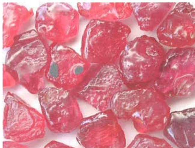
Rubies covered by colorless lead rich glass after heat treatment in Chanthaburi.
