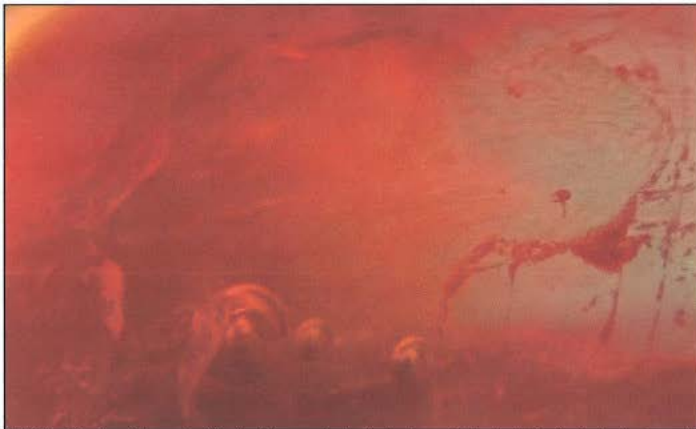
Figure 13: The identification of large glass filled cavities can also be challenging as the lead glass' refractive index is very close to the host's refractive index and the difference in luster is not obvious as shown here. Nevertheless in this example large gas bubbles are useful evidence to properly identify the presence of the glass filled cavity. However, this sample also shows that polishing has damaged some areas where the glass meets the ruby. Photo: V. Pardieu
