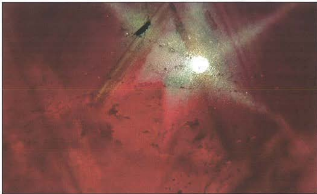
Figure 10: The identification of the flattened gas bubbles is challenging due to the presence of dense silk. Photo: V. Pardieu
