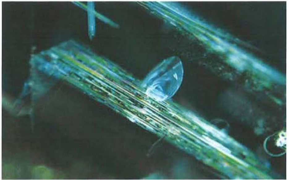
Figure 5: A more recent type of heated spinel encountered by the AGL revealed thermally induced inclusion features more consistent with what may be seen in rubies and sapphires heated to relatively lower temperatures. These included disoid or atoll-like induced stress fractures with a partial healing rim as seen extending from needle-like inclusions. (Photomicrograph: Christopher P. Smith, 75x)
