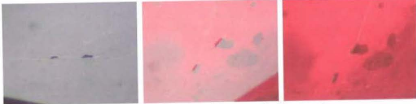
A wide fissure filled with lead glass from a Bangkok repaired ruby presents a noticeable orange color. Left to right: overhead, transmitted and dark field illumination.
