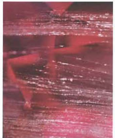
Figure 4: Concentrations of fine stringer-like inclusion features are common to certain sources of spinel. In the heated spinels submitted to the American Gemological Laboratories (AGL) to date, such stringer-type inclusions revealed an atypical or disturbed appearance. (Photomicrograph: Christopher P. Smith, 42x)
