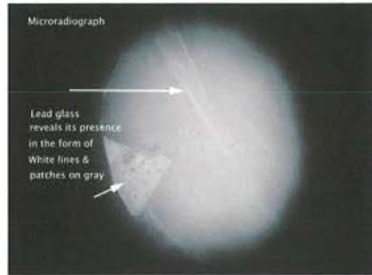
Figure 1b: A microradiograph that reveals the presence of lead glass in fractures
