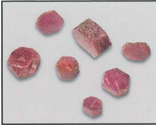
Figure 3: Low-quality rough ruby, commonly from Madagascar, is the starting material for the lead-glass treatment. After the multi-step treatment process, the transparency and color of stones such as these becomes dramatically improved. Photographs by Fred Kahn and Sun Joo Chung.
