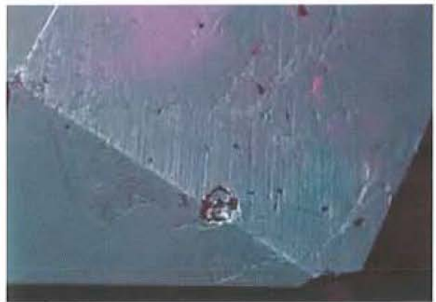
Figure 14. Glass, particularly high-lead-content glass, is significantly softer than corundum, so sometimes the best way to notice a glass-filled cavity in reflected light is by the poor polish on its surface. Photomicrograph by C. P. Smith; magnified 45 \times .
