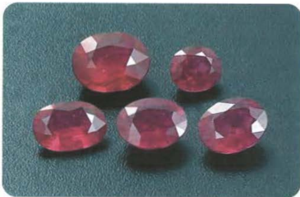
Figure 1. These stones (2.15–7.42 ct) are typical of the final result achieved with the filling of fractures in rubies with high-lead-content glass. Photo by Elizabeth Schrader.
