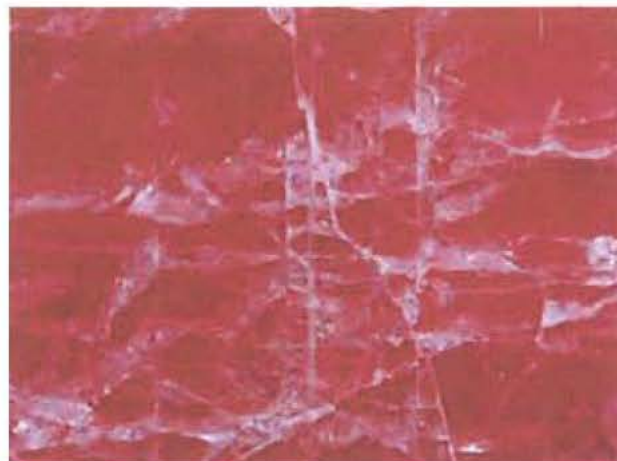
Figure 25. Ammonia, bleach, and even concentrated lemon juice damaged the lead-glass filler at the very surface, producing the whitish areas shown here. Photomicrograph by C. P. Smith; magnified 32 \times .
