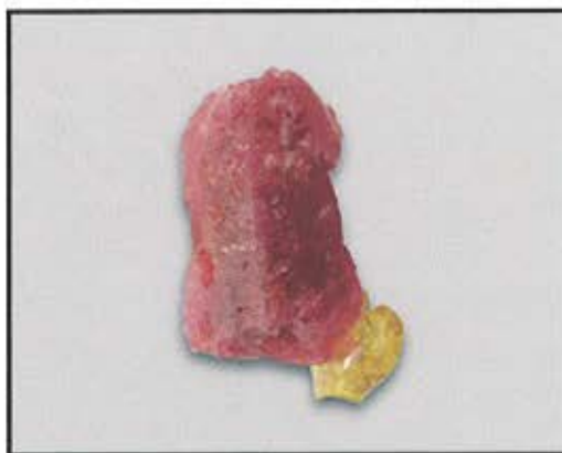
Figure 5: A large piece of the yellow to orange colored lead-glass used in this treatment process can be seen still attached to this large piece of ruby rough after the treatment has been completed. The inherent color of the glass helps to artificially augment the red color of the ruby. Photograph by Fred Kahn and Sun Joo Chung.
