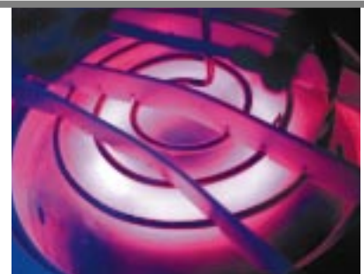
Fuji Electric developed a system that uses induction coupled (IC) plasma to reduce the weight and volume of ion-exchange resins. Although these resins are used in large volumes at nuclear plants and other facilities, a suitable method for processing the used resins has not been established. We expect our new volume-reduction system to solve this environmental issue.
