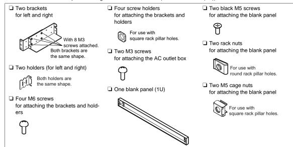
\*4: Confirm that there are no parts missing from the rack mount kit (for AC outlet box (2U)).
