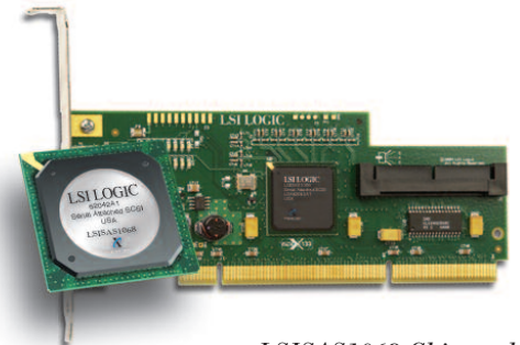
LSISAS1068 Chip and LSI Logic SAS3442X-R Adapter Board
