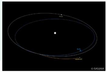
The orbit of Hayaubsa2, going away from the orbit of the Earth after the Earth swing-by
