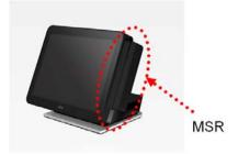
2. Move the magnetic stripe card in the direction of the arrow. Move the magnetic card from the far end of the slot to the front.
