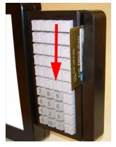
**NOTE:** The MSR reader may not be able to read the magnetic stripe card correctly if the movement of the card is stopped midway, if the card is not moved at a constant speed, or if the card is not moved parallel to the slot.
