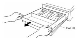
• To insert the cash till into the drawer, open the drawer completely. Then, perform the above steps in the reverse order.
