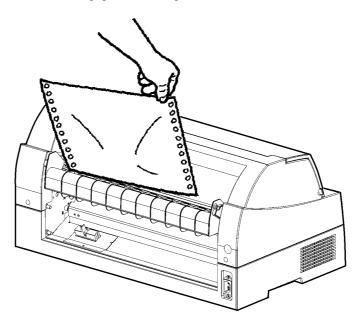
Tearing off continuous forms (front feed)
