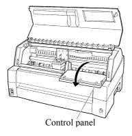
Preparing the printer to install the ribbon cartridge
