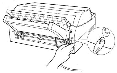
5. Extend the extension and extension wire in the order from (1) to (2) according to the size of the paper to be used
