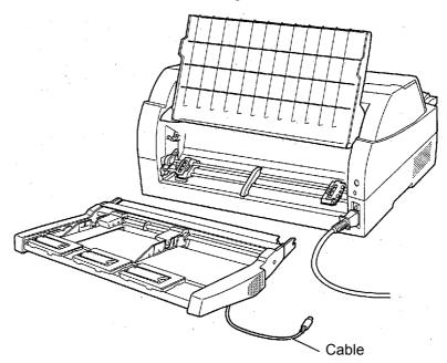
When mounted on the rear side of the printer
