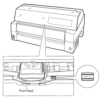
Adjusting Load Position by Using Window of Card Guide
