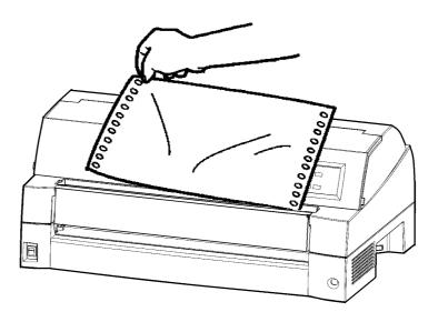
Tearing off continuous forms (rear feed)
