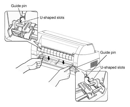
3) Verify that the hooks on both sides of the tractor unit are securely hooked onto guide pin 2 as shown in the following figure.
