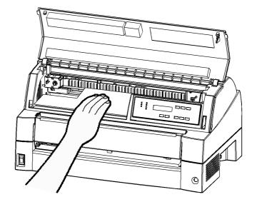
Removing the shipping restraint cardboard
