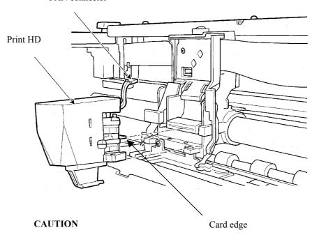
Be carefully to remove the card edge and FAN connector straightly.
