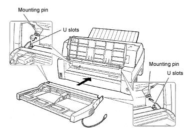
Check that the cut sheet feeder frame is correctly mounted on mounting pin 2.
