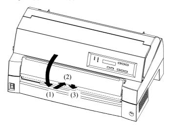
The complete setup conditions are shown below. Make sure that the top end of the soundproof cover is engaged with the printer guide pin and the guide pin on the soundproof cover is inserted into the cover groove.
