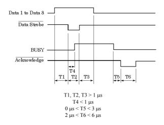
In bidirectional mode (nibblemode), this printer can send data to the computer. Data is sent in units of four bits (nibble) using four output signal lines as data paths. The following outlines one byte of data sent during reverse data transfer phase in nibble mode.
