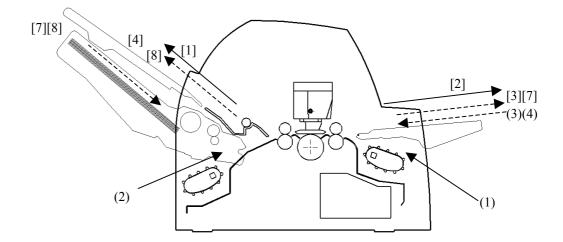
With rear tractor and front and rear optional cut sheet feeder and large stacker and large paper table.
