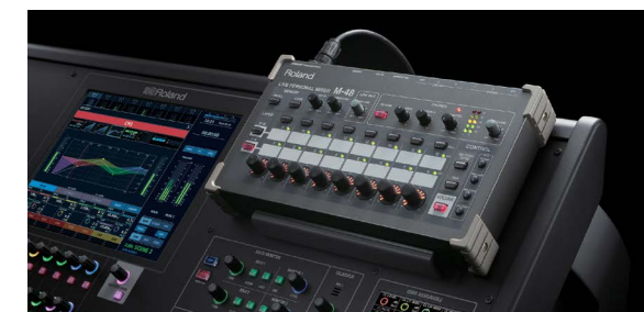
M-48 Personal Mixer being used as an Engineer's Monitor, powered by the Backup port
