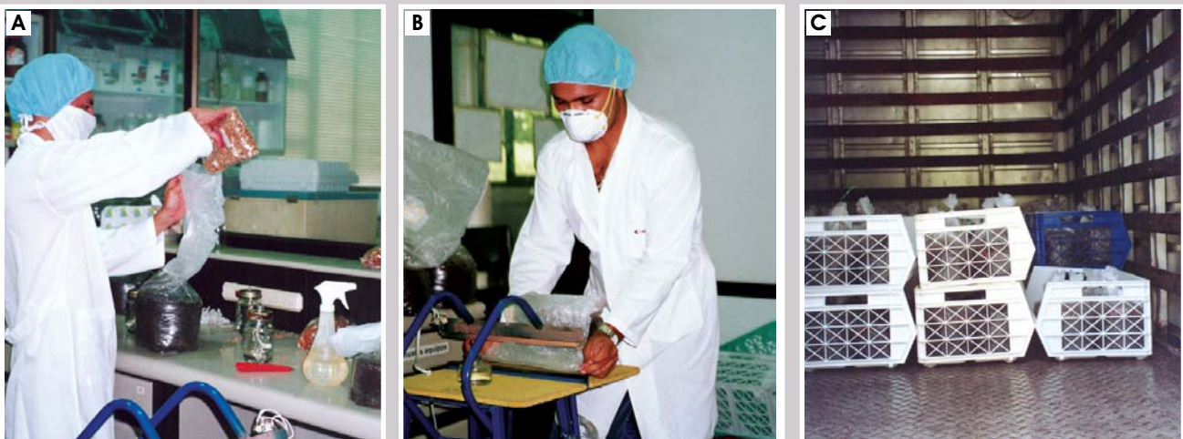
Figure 10. Central production of inoculated substrate bags A: Spawning (grain spawn) B: Heat sealing of the bag C: Inoculated bags in the truck ready to be delivered to growers
