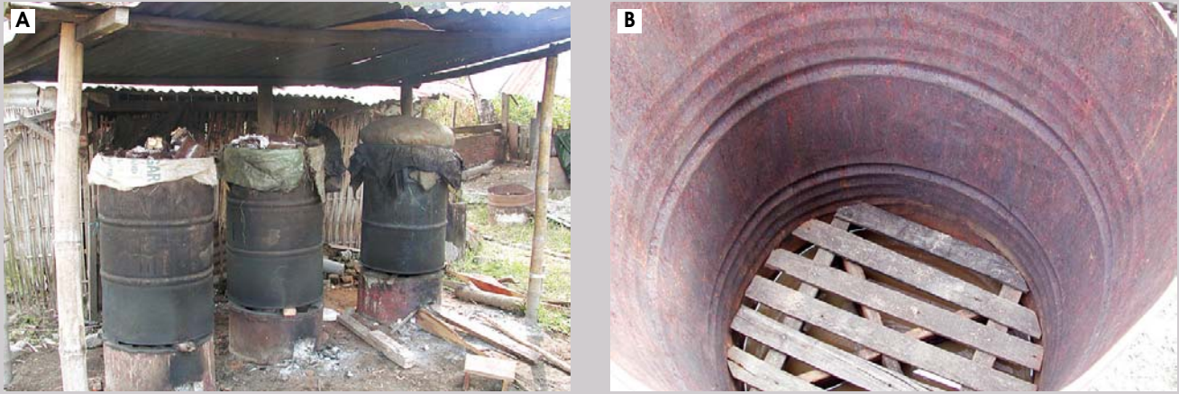
Figure 10. Drums for pasteurization A: Drums on fireplace B: Rack inside the drum
