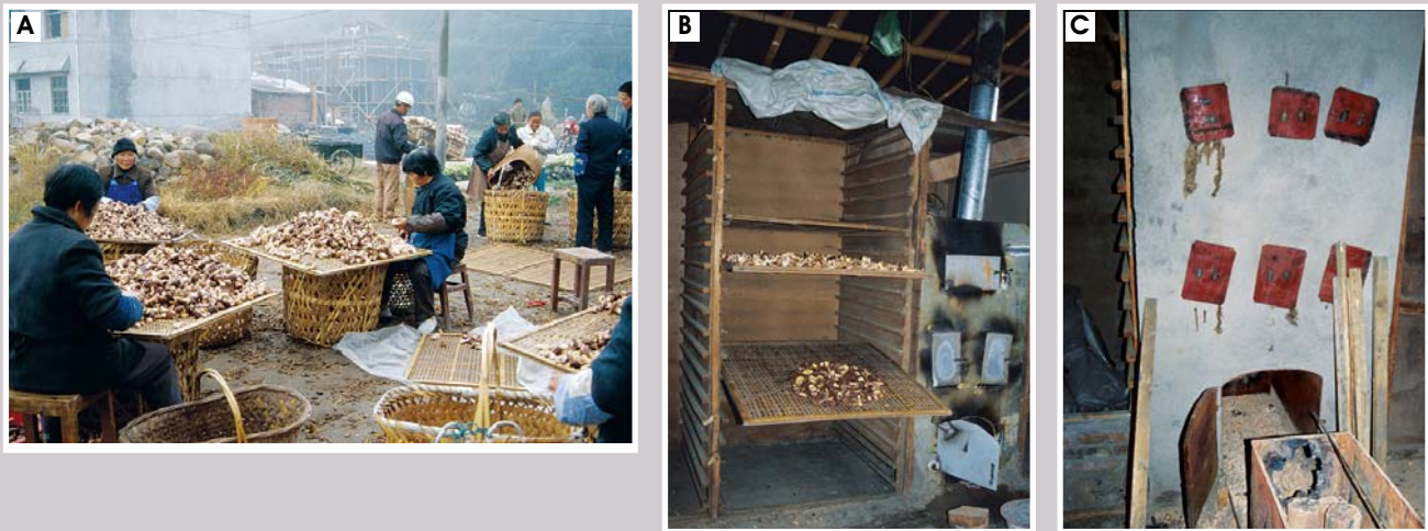
Figure 12. Trimming and drying shiitake A: Trimming and grading shiitake before market delivery B and C: Drying equipment using hot air and its fire place
