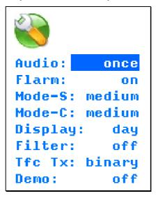
The desired menu item can then be selected by one or multiple presses of the minus key . Selection goes repeatedly from top to bottom. The blue background indicates the active menu item that can be adjusted with the key. More details on each menu item can be found in the following segments.
