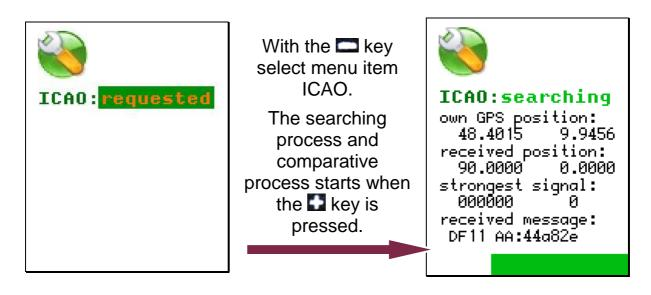
After a successful comparison, the recognized ICAO 24-bit address will be displayed.
