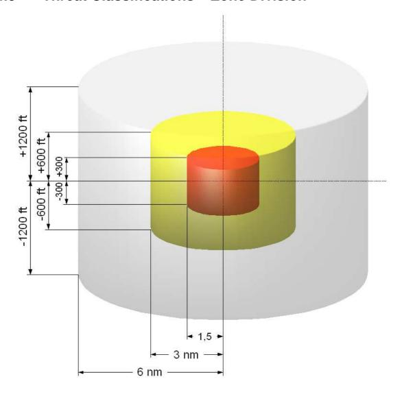
Basically, the collision warning is based on the comparison of the own position with the location of surrounding traffic. With ADS-B traffic, this is done using the respective position reports. For Mode S traffic (not ADS-B capable), the field strength is measured. The proximity of FLARM<sup>®</sup> traffic is detected whenever a signal is received (which suffices as the maximum range of FLARM<sup>®</sup> reception is relatively small).
