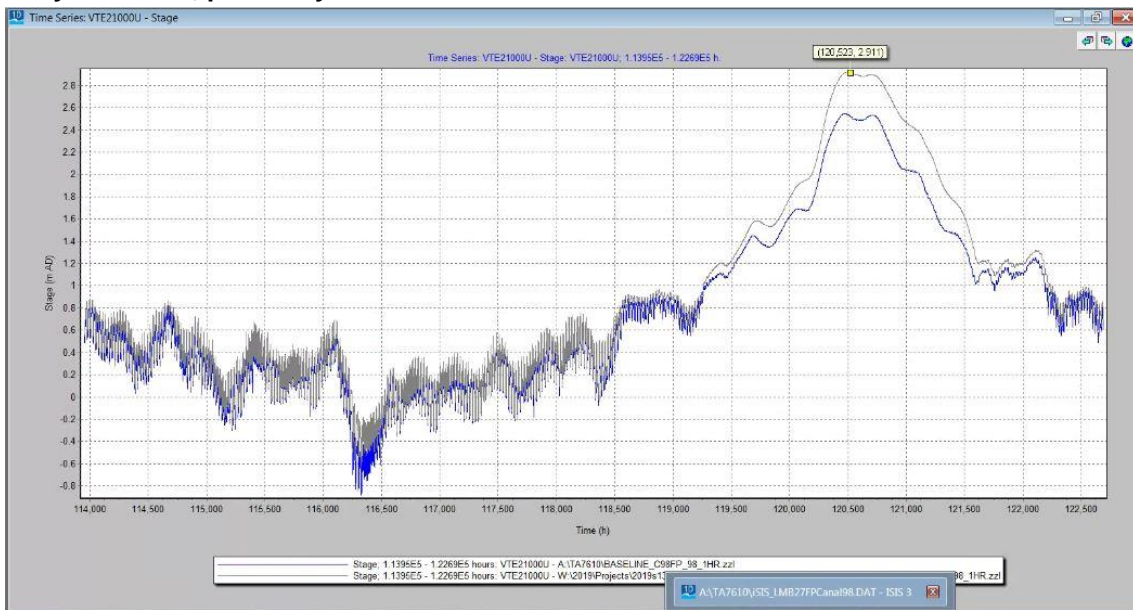
Figure 6-5: Water Level at Road at border with and without flood protection (1998 dry year)
