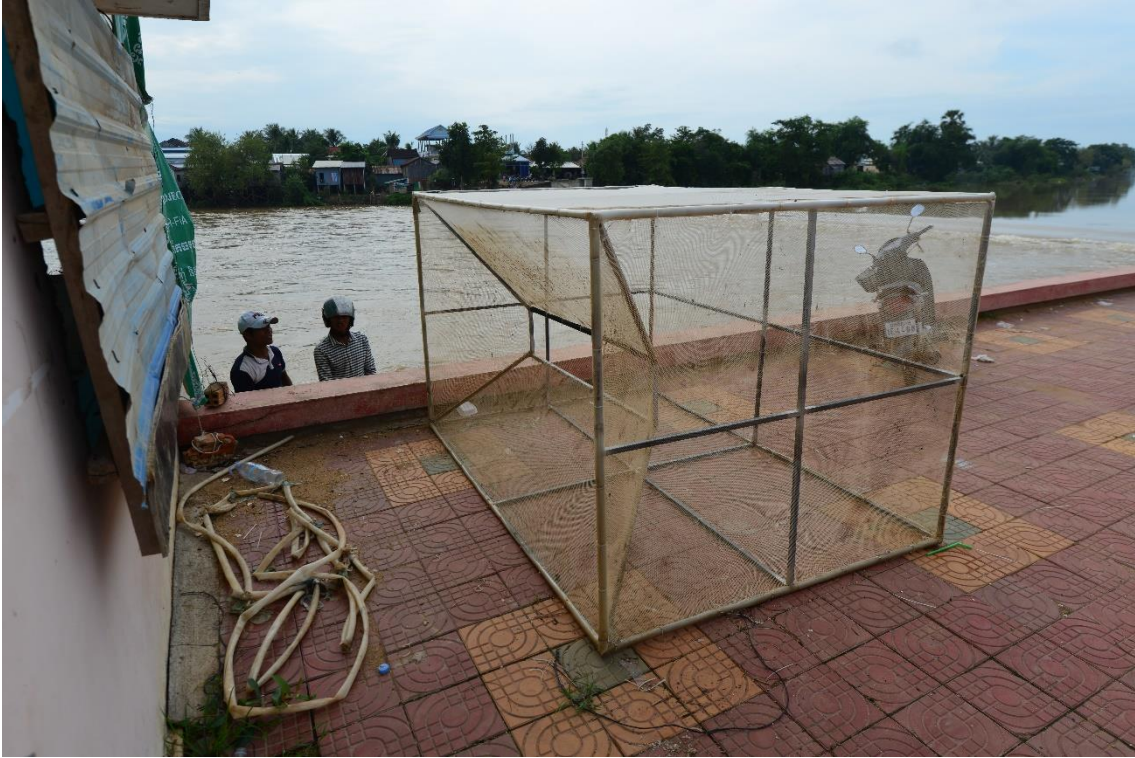
Photo 9: Trap used to monitor fish passage in Kbal Hong fish-pass
