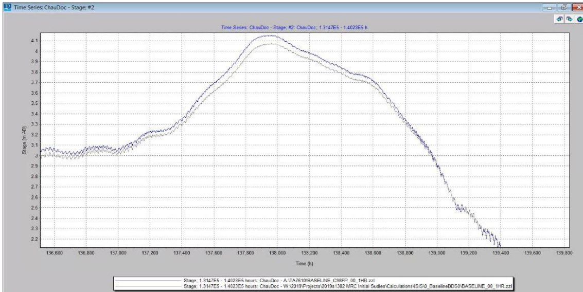
Figure 6-4: Water Level at Chau Doc with and without flood protection (2000 wet year,) full year above, peak only below.
