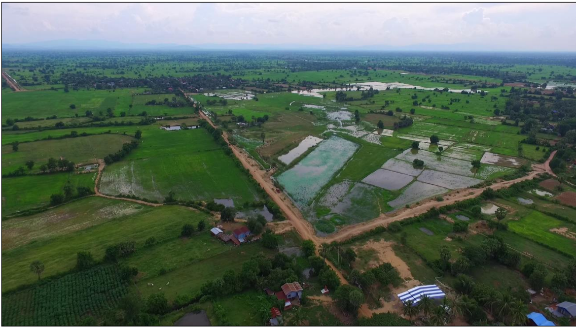
Photo 36: Ang Ta Nak CFR, opposite view Road levees dam the drainage line and also off the CFR, culverts were installed later
