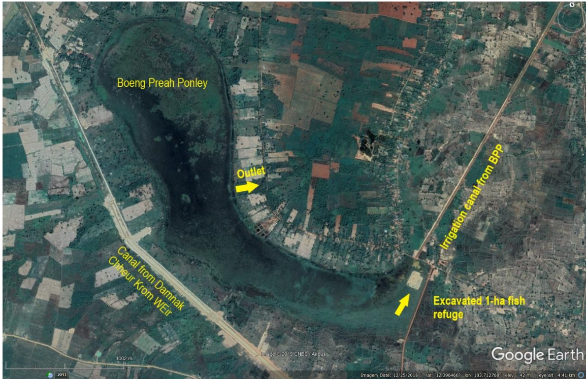
Photo 25: Boeng Preah Ponley, a 2600-ha natural wetland on 25/12/2018 The canal from Damnak Chheur Krom reportedly cut off some overland flow to the lake. The lake is shallow and overgrown by aquatic weeds. A dry season fish refuge of 1 ha was cleared of plants in the northern section in 2014, but the plants quickly regrew. A 1-ha fish refuge was excavated near the main wall in 2018.
