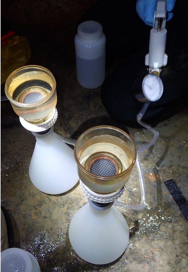
Figure 1. – Filtration setup for eDNA collection. Two, 1-L water samples were collected from each sampling unit. While wearing nitrile gloves, a 0.45- \mu\text{m} microbial filter was placed inside a filter funnel that was attached to a vacuum flask via a rubber stopper. A hand pump was used to create a vacuum and pull water through the filter. Filters were stored in 900 \mu\text{l} of Longmire’s buffer (Longmire et al. 1997).
