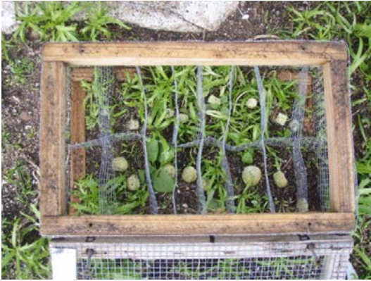
Fig. 1 Photo of bait degradation cage with pellets. Wire mesh bottom on this cage not visible in picture.
