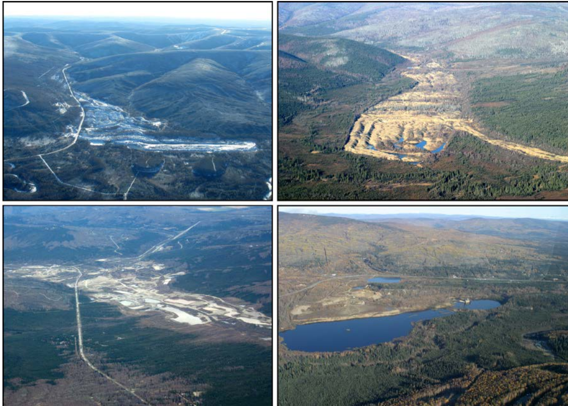
Figure 59. Tailing piles and dredged regions in lower Cleary Creek in the Chatanika River drainage (upper left), Fairbanks Creek in the Chena River drainage (upper right), Goldstream Creek at the community of Fox (lower left), and Ester Creek near the community of Ester (lower right). The dredged region in Cleary Creek is adjacent to a major whitefish spawning area on the Chatanika River (Kepler 1973), which is visible in the lower corners of the image. The dredged region across the Fairbanks Creek floodplain has created an isolated population of Arctic grayling upstream, because the stream now flows subsurface through the extensive tailing piles (Ott and Townsend 1996; Morris and Ihlenfeldt 2008). Photos by R.J. Brown, USFWS.
