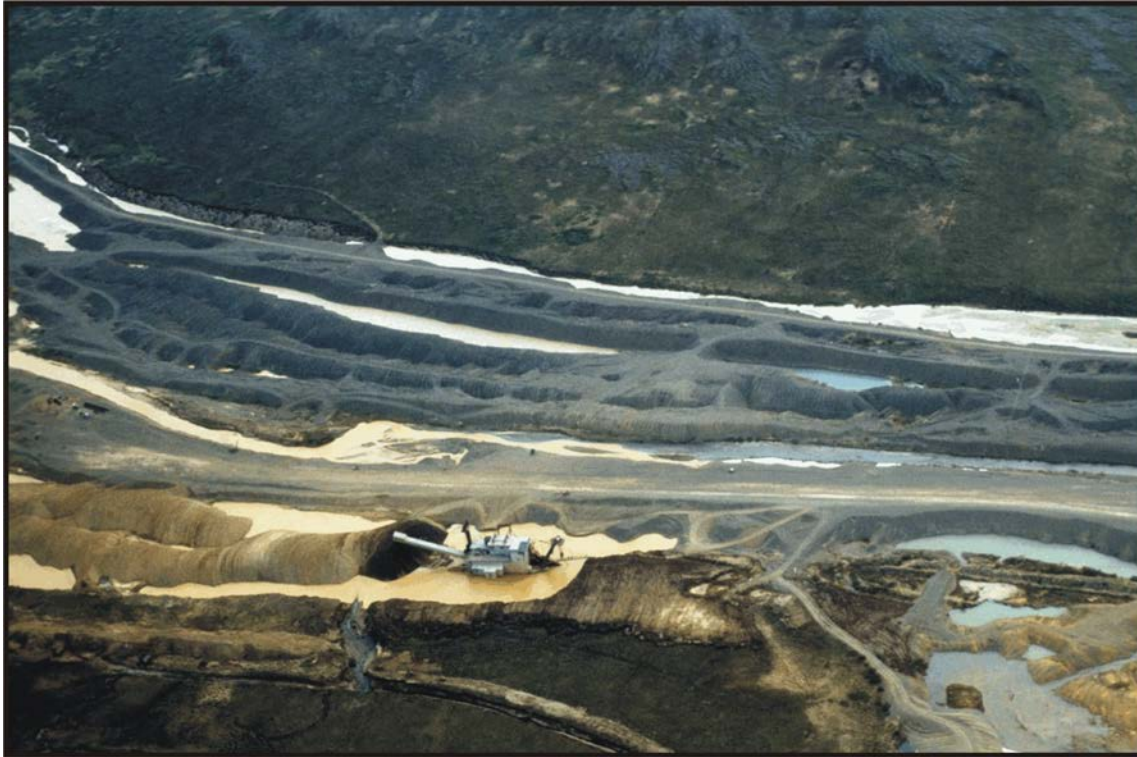
Figure 94. A 1972 photograph of a large floating dredge working the platinum mine on the Salmon River just south of Goodnews Bay in southern Kuskokwim Bay. It should be noted that floating dredges have worked over most of the Salmon River valley and several of its tributaries, creating a nearly drainage-wide network of tailing piles similar to the image above. Photo by USFWS staff.
