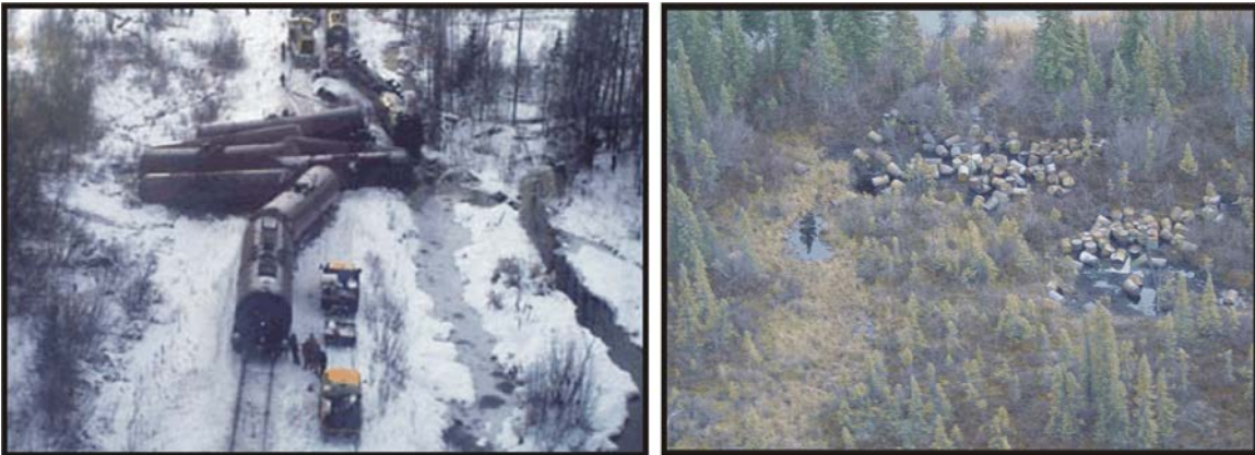
Figure 18. Aerial images of two common types of industrial fuel spills. On the left is an Alaska Railroad derailment of fuel cars in which a large quantity of fuel was spilled (photo courtesy of the Alaska Department of Environmental Conservation). On the right is a photograph of a cache of leaky fuel barrels on Billy Hawk Creek, a tributary stream within the Koyukuk River drainage. These barrels, which contained diesel fuel, had been left at the site for over 40 years before their discovery in 2002 by residents of Huslia (photo by USFWS staff).
