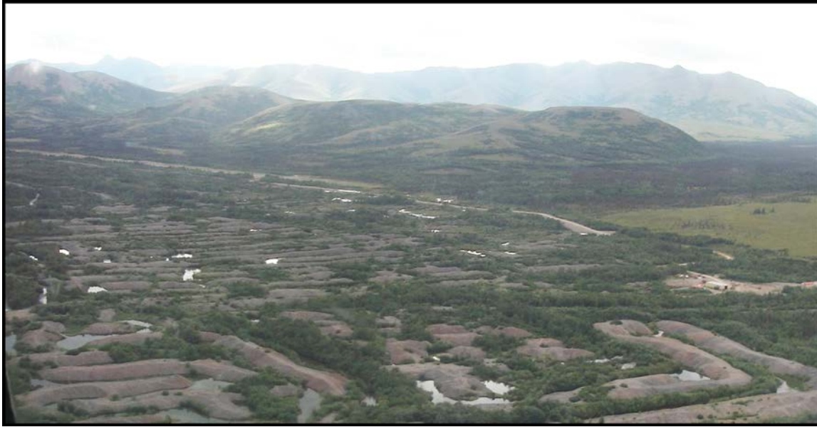
Figure 88. Tailing piles extend completely across the upper Tuluksak River valley at the Nyac mine. A segment of the valley more than 15 km (10 miles) long was extensively dredged beginning in the early 1900s, which repeatedly rerouted the natural river course. The river now flows around and through the maze of tailing piles. Any critical fish habitat that may have existed before the mine was active has been irrevocably altered. Photo by K.C. Harper, USFWS.
