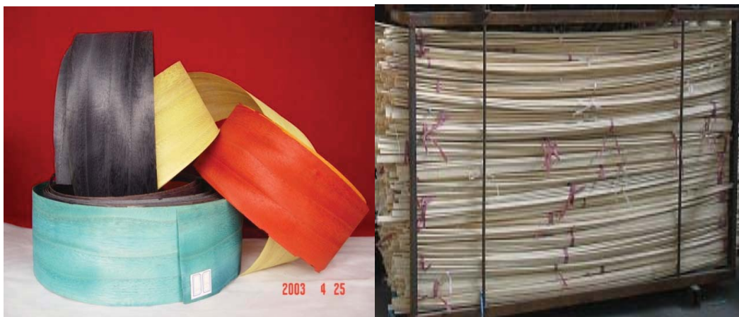
No. 3 of 10 series of bamboo products: Bamboo rotary-cutting veneer and its dyeing and bleaching
