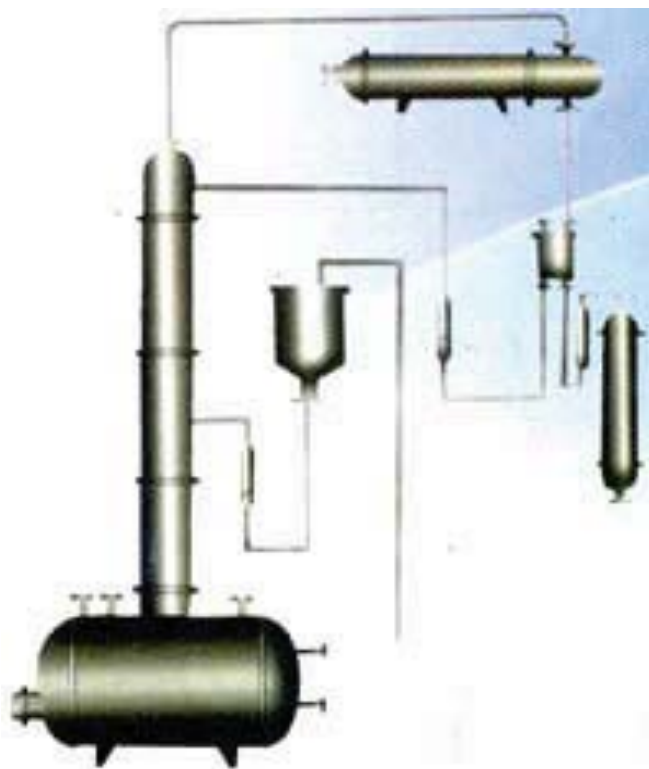
Fig.2 Normal Atmosphere Distillation Device
