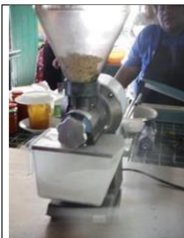
A small grinder for manufacturing breadfruit flour at the Tutu Rural Training Center, Taveuni Fiji
