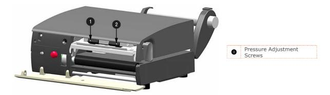
5. Re-latch the printhead and repeat the test print. Repeat step 4 until an acceptable print has been achieved.
