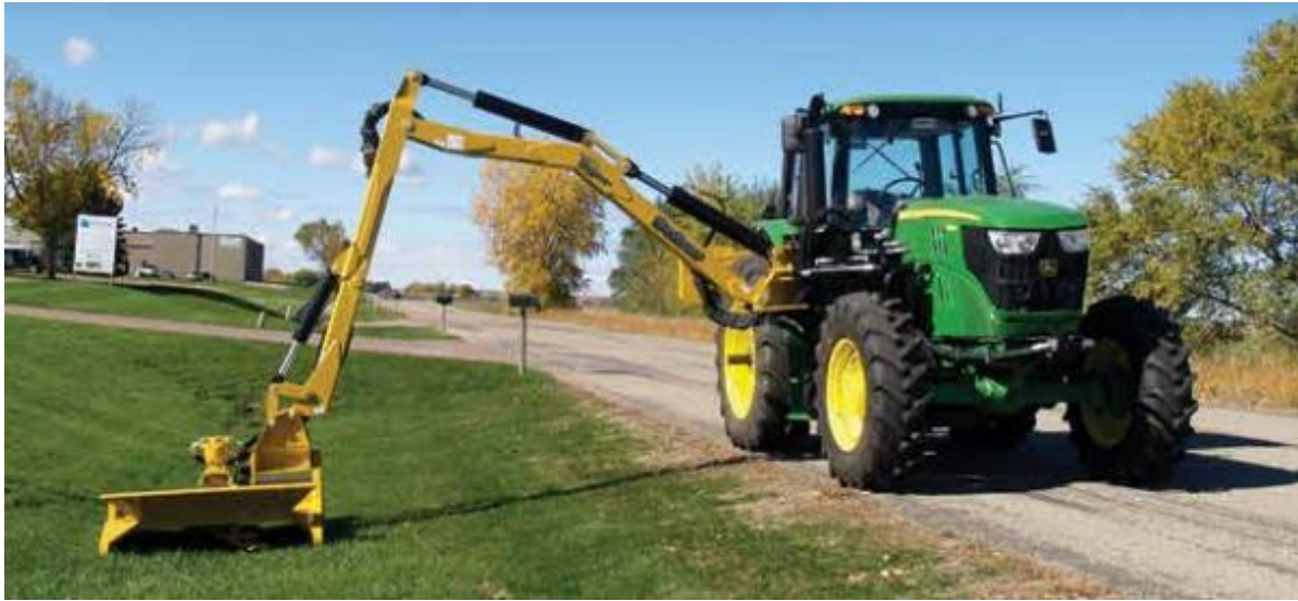
Above: Flail mower on an articulated arm capable of adjusting deck angle to match terrain (chattanoogatractor.com).
