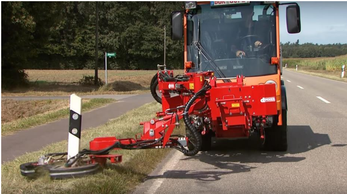
Above: Articulated mower with deck which pivots around roadside posts, improving mowing maintenance efficiency and verge coverage.
