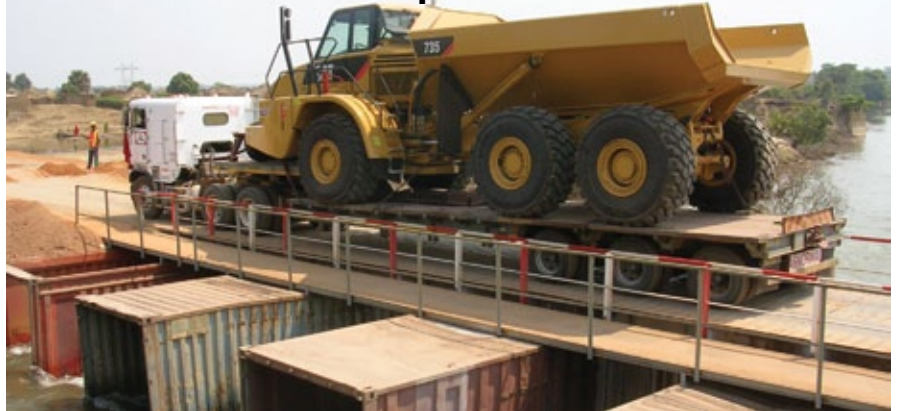
A flatbed hauls an articulated haul truck across a bridge constructed from freight containers. Photo courtesy of Congo Equipment.
