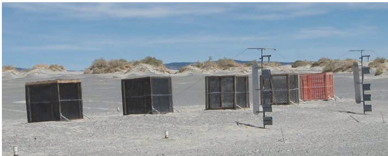
FIGURE 4-11 Testing of engineered porous roughness elements at Mono Lake. SOURCE: Holder, 2019c.
