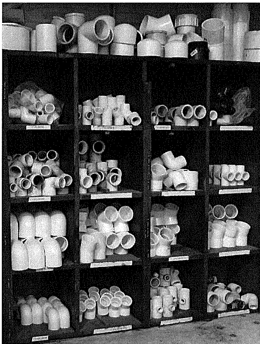
A selection of pipe fittings and repair couplings of different sizes should be on hand so that repairs can be made in a timely manner.
