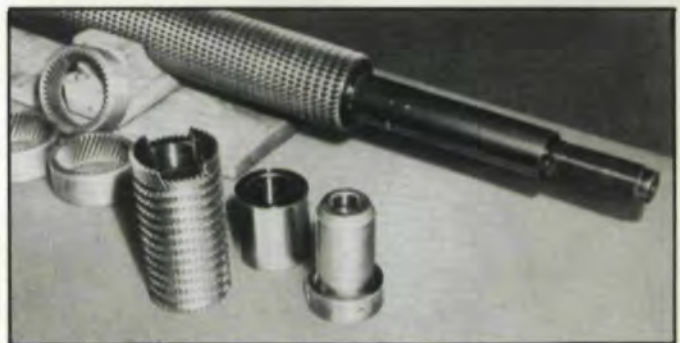
Fig. 10—Full-form finishing broach showing roughing section, finishing shell, tailpiece and broached gears.
