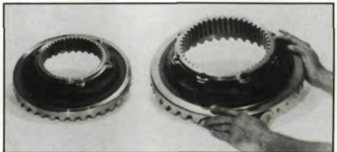
Fig. 14—Large internal spur differential running gears that are broached to precision tolerances.
