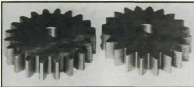
Fig. 6—Hobbed 4-DP, 5-in. PD, 20-tooth gears with 20°-PA, left, and 30°-PA, right.
