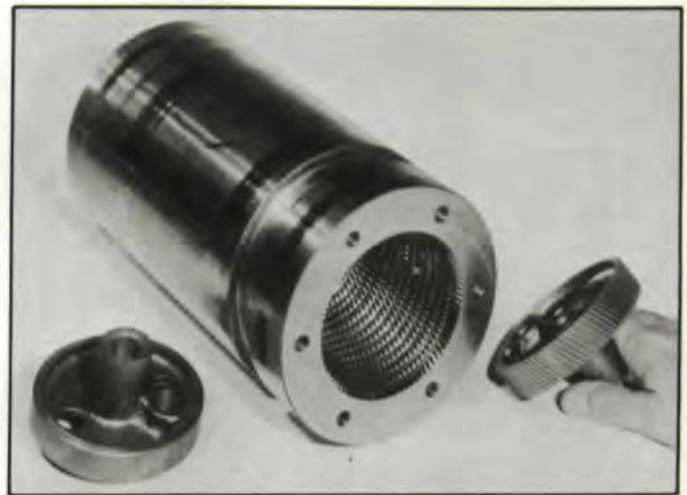
Fig. 17—A solid HSS pot broaching tool that produces external helical cast iron running gears.
