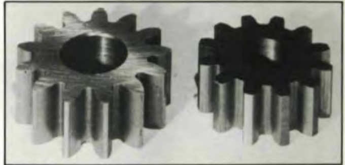
Fig. 8—Gear-Shaped 5-DP, 20°-PA, 13-tooth gear, left, produced by a 20-tooth, 4½-in. OD shaper cutter; compared with a 5/7-DP, 20°-PA, 12-tooth gear, right, produced by a 15-tooth, 3.325-in. OD cutter.
