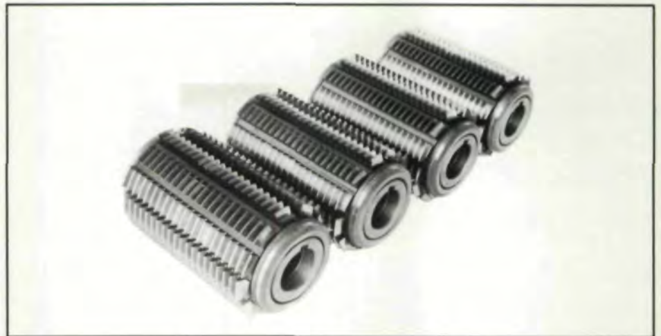
Fig. 9—Multi-thread hobs with small diameter
