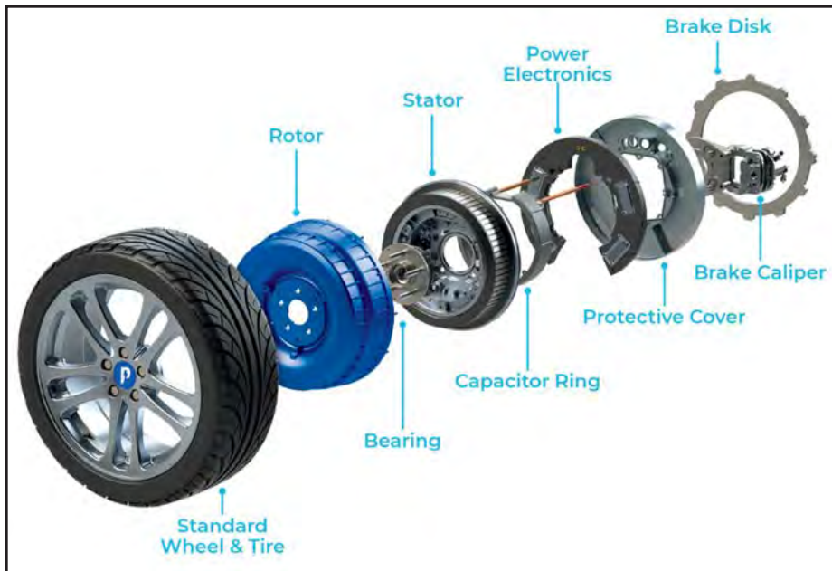
Figure 10 In-wheel direct drive motor (Ref. 10).
