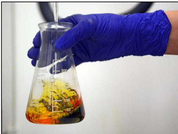
Figure 4 By monitoring the acid level, the oil can be changed before any damage occurs; an oil analyst is looking for a sudden increase.
