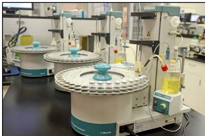
Figure 6 If a crackle test is positive, further testing is needed to quantify the amount of water by using Karl Fischer titration by ASTM D6304 (ASTM, 2007).
