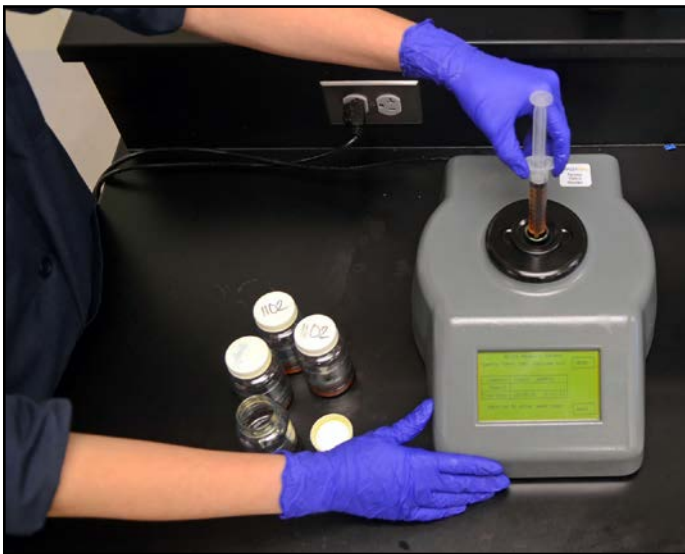
Figure 8 A wear particle analyzer quantifies the amount of ferrous material present in a sample of fluid.
