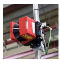
application technology enable high coating quality for the 53 color shades and 17'000 programs, which are stored in the data base. Laser scanners are detecting the part geometry and control fully automatically the individual horizontally moving gun axis. This guarantees the effective coating of difficult part geometries in highest quality.
