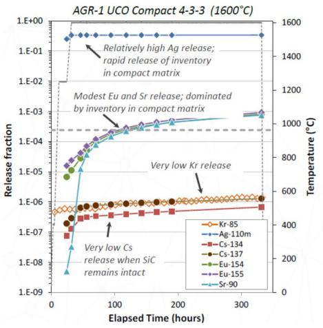
AGR TRISO fuel has successfully survived 300+ hour safety tests at 1600 C, 1700 C, and 1800 C.
