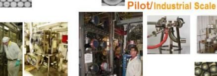
Industrial Scale 6 inch CVD Coating (2 kg charge)
