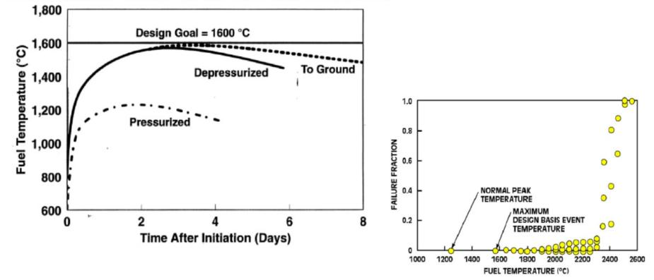
The multilayer TRISO coated particle fuel is engineered to retain fission products during normal operating conditions (~1000-1400 C) and all gas reactor licensing design basis accident events (~1600 C), including a Depressurized Cooldown Event (loss of coolant), the worse event for a HTGR.
