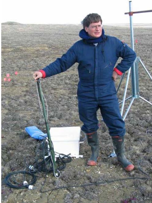
Figure 4. (a) Valdimir Romanovsky installing a climate station at the zonal grid site. The tripod behind him holds a sonic snow meter, solar panel, and air temperature sensor. The probe he is holding was buried in the soil, as shown in photo (b), and measures temperature and moisture at depth.
