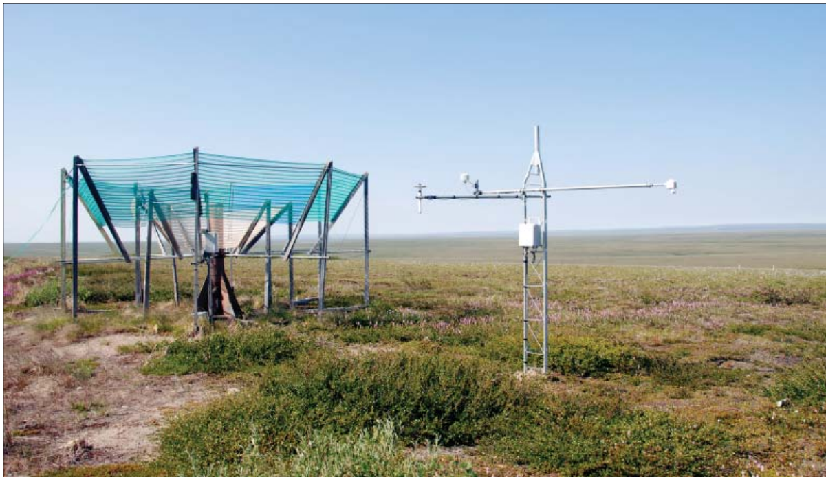
Figure 48. Wyoming snow gauge and climate monitoring site at Sagwon. Photo by D.A. Walker.
