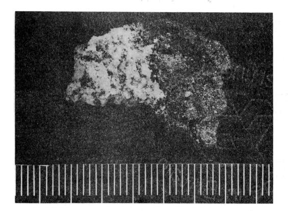
Fig. 2 White efflorescent decay products on pyrite sample from Nenagh (Scale in mm.)
