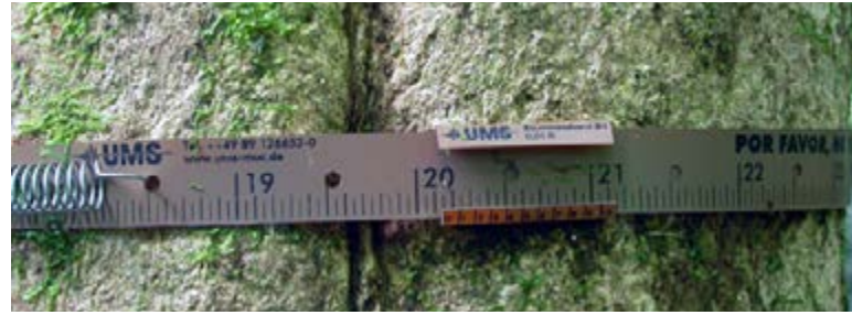
Figure 6: Dendrometer tapes measure the stem diameter increments at breast heights (dbh). Photo: J. Homeier
