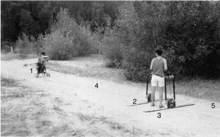
Fig. 8. PulseEKKO IV GPR field system outfitted with 50 MHz antennae set up for profiling: console and display unit attached to golf cart (1); transmitter antenna (2); receiver antenna (3); fibre-optic cable (4); survey line (5).
