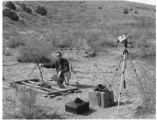
Fig. 3. GPR on wooden cross-beams inside the frame.
