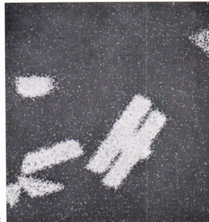
Fig. 3. Sb-westerveldite (1), seinäjokite (2) and tellurides in native antimony. 3-altaite; 4-non-determined telluride; 5-pyrrhotite. Magn. 700x. a — back-scattered electron image; b — SbL_{\alpha_1} X-ray image; c — FeK_{\alpha_1} X-ray image.
