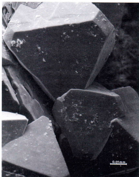
Fig. 4. Euhedral pyrite crystals with (100) and (111) of a miarolitic cavity of drill core Y8, depth 180.86–180.88 m. Scanning electron microphotograph by B. Johanson.
