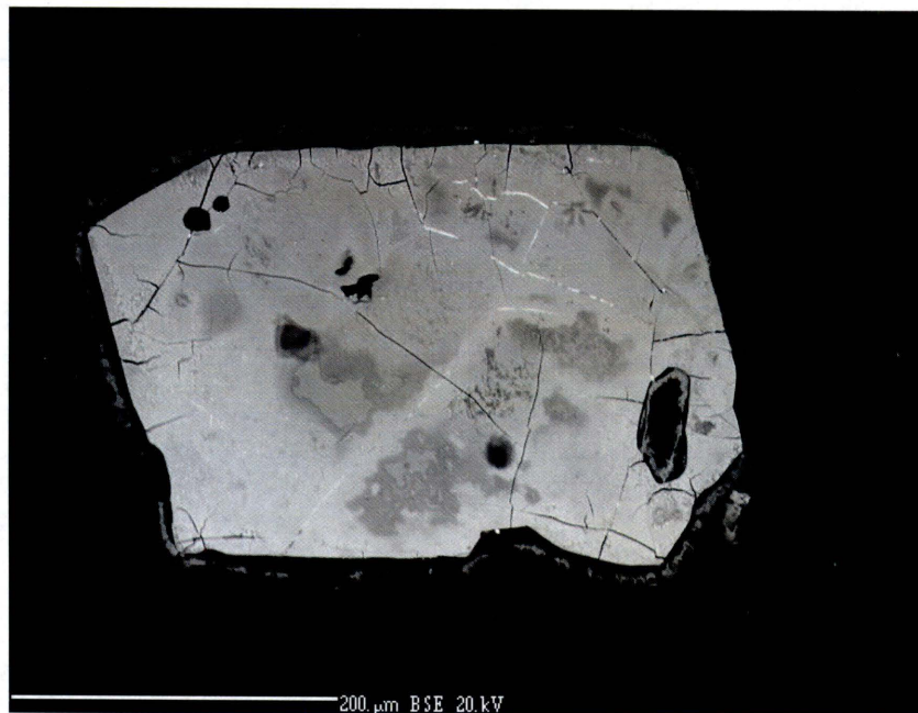
Photo 11. Pyrochlore grain from silicocarbonatite zone in sample 26380 that shows patchy zonation and late crosscutting veins with a bright white mineral that could not be identified but possibly a REE phase. Lighter areas contain elevated BaO and SrO vs darker patchy remnants.
