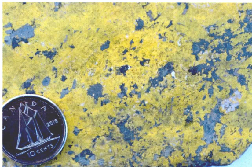
Photo 4. Leucocratic syenite segregation of hastingsite-magnetite-diopside-Ba-rich K-feldspar (yellow stain): 26362
