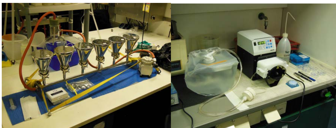
Fig. 8.2: Filtration plant set-up for water samples to determine chlorophyll a and silicate in shipboard wet chemistry laboratory, filtration device for coccolithophore filtrations samples in the background (left). Peristaltic pump set up for suspension filtration of IOW water samples (right).
