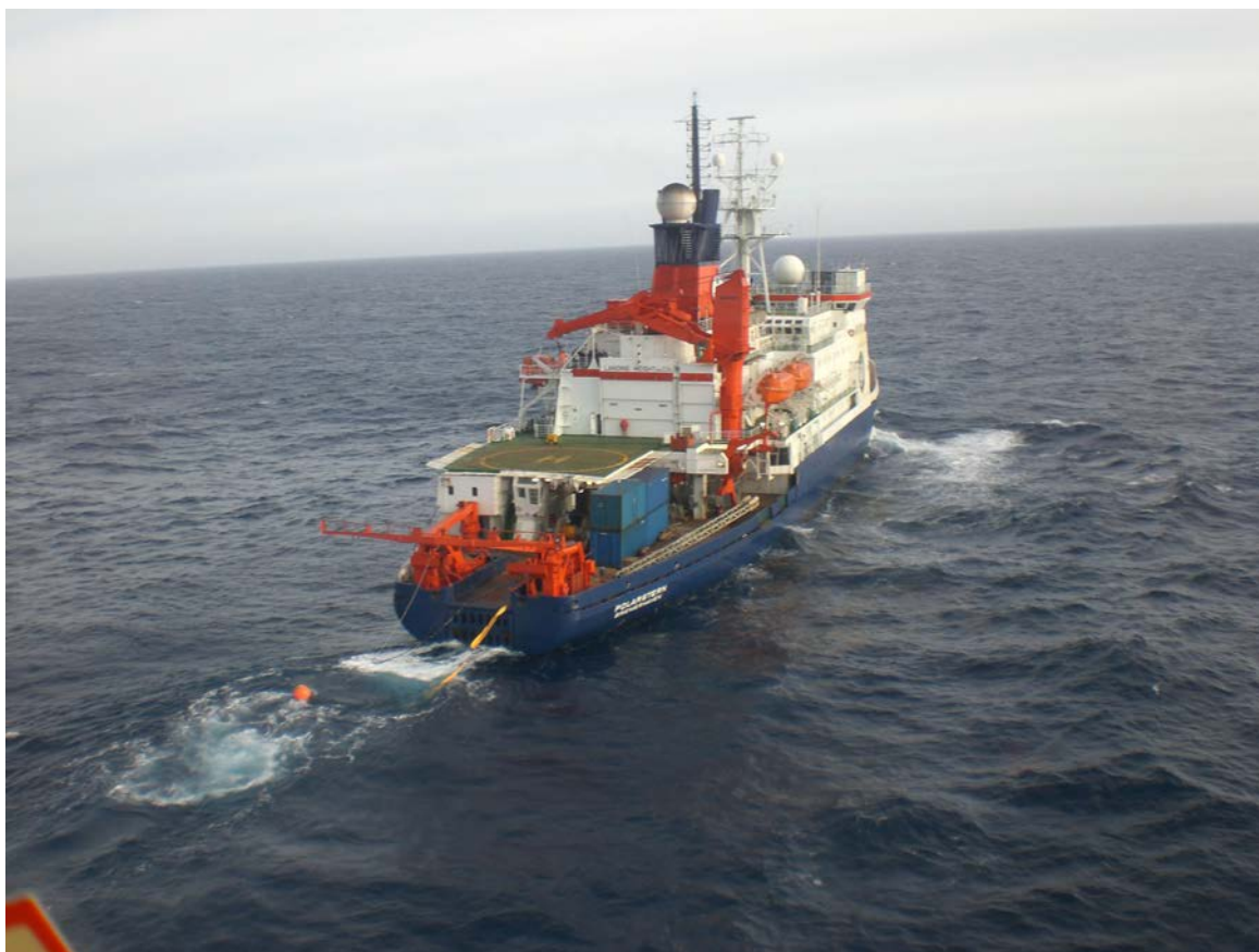
Fig. 6.3.4: Photo of RV Polarstern with the towed airgun and 600 m multi-channel streamer (Photo: ?).
