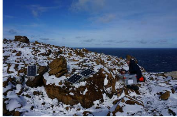
Fig. 4.4.4: Installation of the GPS equipment at the sites ELE1. The left photograph shows mounted GPS antenna on the existing GAP marker from 1995. The right photograph shows the solar-panels (left) for power supply of the receiver and the Zarges aluminium box (right) to protect the receiver and battery.
