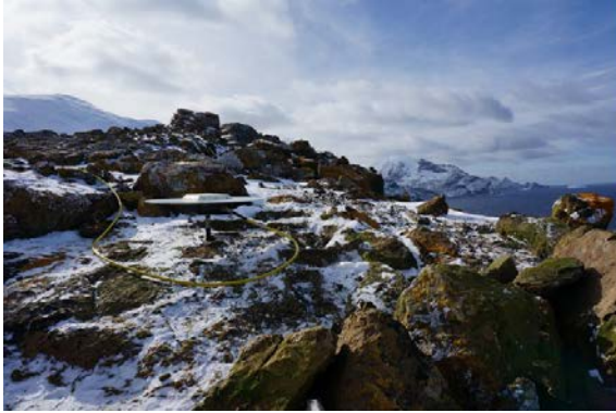
Fig. 4.4.4: Installation of the GPS equipment at the sites ELE1. The left photograph shows mounted GPS antenna on the existing GAP marker from 1995. The right photograph shows the solar-panels (left) for power supply of the receiver and the Zarges aluminium box (right) to protect the receiver and battery.
