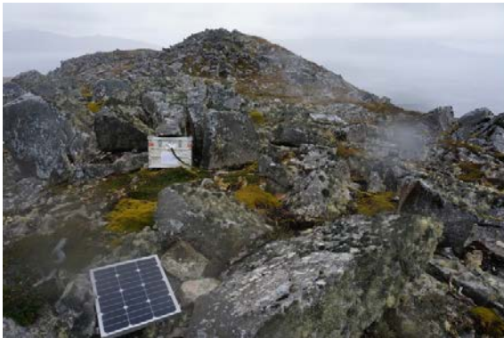
Fig. 4.4.5: Installation of the GPS equipment at the sites HORN. The left photograph shows a solar panel and the aluminum box (the middle ground). The right photo shows the mounted GNSS antenna.
