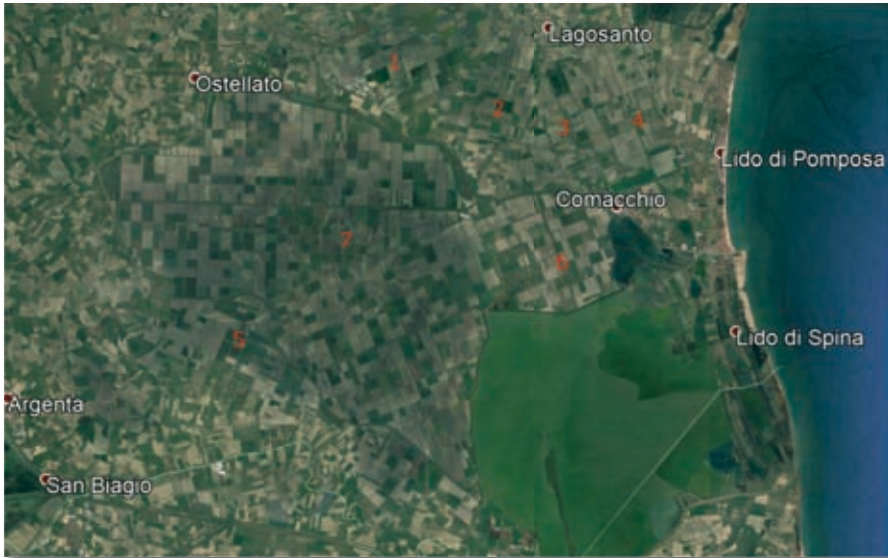
Figure 3. The present-day situation of the Emilia-Romagna sector of the Po River Delta: a man-made delta, where most of the original wetlands have been artificially drained and turned into fields, now organized on the basis of a perfect square grid. The reclamations of the former wetlands of Figure 2 are highlighted with the same numbers in the satellite image; on the right, is the small sector of the wetlands of the Po River Delta, which survived the reclamation programme (source: Google Earth).
