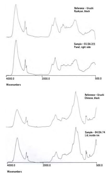
Figure 2. Infrared absorbance spectra of two urushi samples. The sample on top is from a Chinese black lacquered food bowl, and the sample on bottom is from the lid of a black lacquered bowl set thought to be of Japanese origin. This visual identification was concurred by computer matching.
