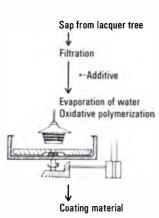
Figure 8. The process of making lacquer from sap, using a vessel equipped with a stirrer.
