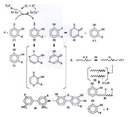
Figure 4. Enzymatic and aerobic polymerization of urushiol.
