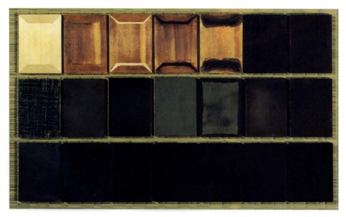
Figure 2. Sample boards showing steps in the process of lacquering, from the basic shape (top left) to the finished product (bottom right).
