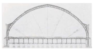
Fig. 49. SAINT PANCRAS STATION, LONDON 1868 Span 73 meters, internal height 25 meters.
