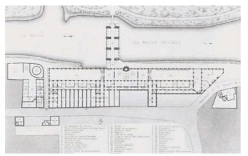
Fig. 41. JULES SAULNIER Menier Chocolate Factory in Noisiel-sur-Marne Plan. The main building on the riverbank dates from 1864-67. The iron-skeleton building shown above is the one that rests on four piers and is set boltlike into the riverbed.
