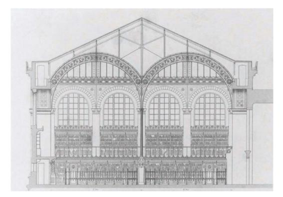
Fig. 12. H. LABROUSTE: LIBRARY OF SAINTE-GENEVIÈVE. 1843–50 Section through the upper story (reading room) and the roof truss.
