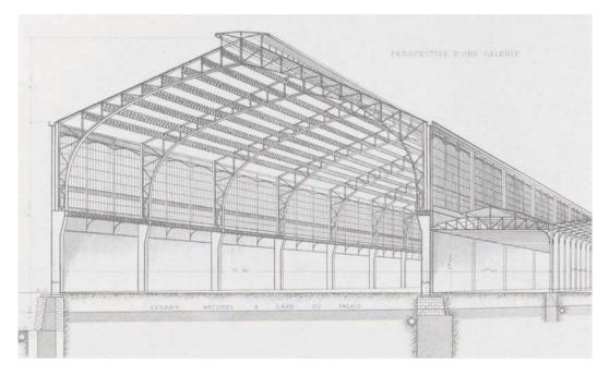
Fig. 47. EXHIBITION, PARIS 1878. GALERIE DES MACHINES. CONSTRUCTOR: HENRI DE DION Span 35 meters. Height 25 meters. For the first time in a large span all the forces connected with the system are carried freely into the foundation without auxiliary means (tie-rod).
