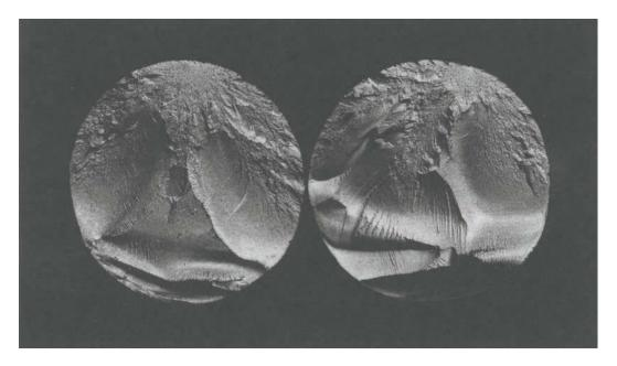
Fig. 5. STEEL. Broken Steel Rod Enlarged Three Times Note the great density of the structure in contrast to other building materials, such as wood: from this molecular structure arise certain properties and types of construction.
