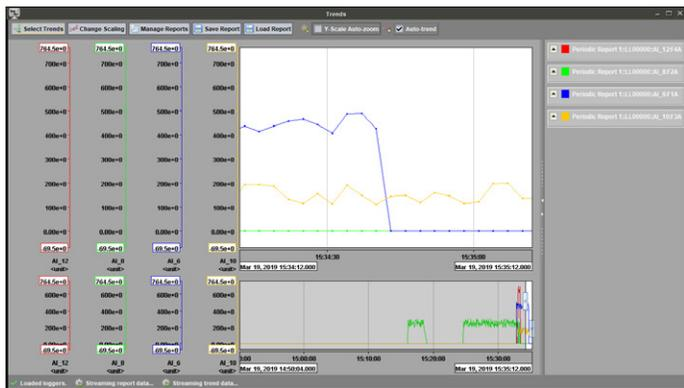
Use device software to obtain non-operational data such as trending and event records through the G100's secure remote access functionality.
