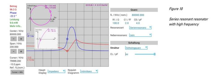
For the following analysis of the resonator quality factor we reset the equivalent parameters of the resonator to the values R1 =  $10 \Omega$ , C1 = 2 fF, C0 = 4 pF.
