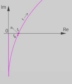
Admittance (left) and impedance (right) of a resonator with higher f requency
