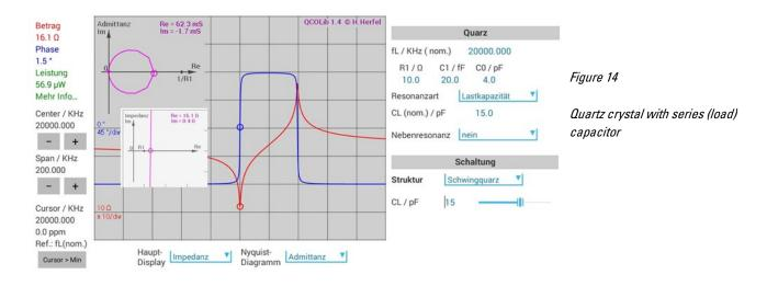
As shown in Figure 14, the distance to the parallel resonance is reduced in comparison to the series resonant quartz crystal (Figure 8). The reason is simple: The load resonant quartz crystal has already been drawn in this direction according to equation 5 with the CL of 15 pF. Shorted series capacitance CL under 'Circuit' thus results again in the old distance from Figure 8 (Figure 15).
