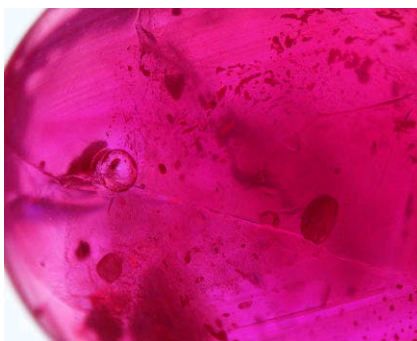
Figure 33. Left: Blue flashes and trapped gas bubbles of various sizes and shapes along surface-reaching fractures and cavities. Field of view 7.64 mm. Right: The bismuth glass-filled fractures and cavities were easily visible in the X-ray image.
