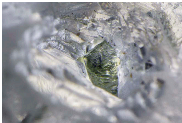
Figure 4. This registered pair of images shows how the green diamond contained inside the negative crystal can change position inside the host diamond and how the green diamond is too large to fit through the opening to the surface. Photomicrographs by Nathan Renfro; field of view 3.20 mm.
