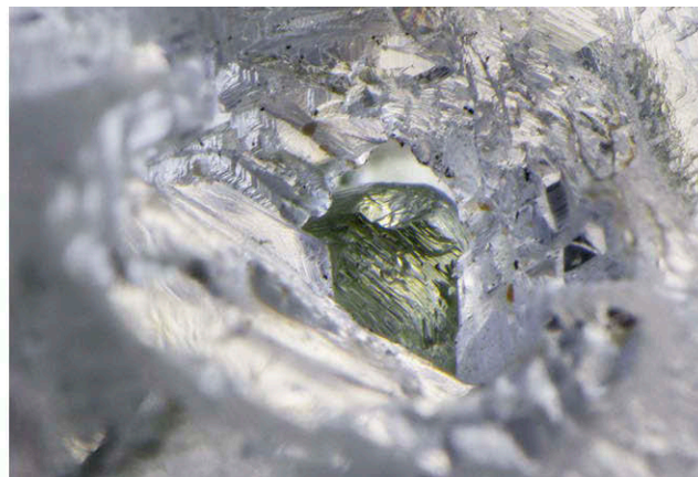
Figure 4. This registered pair of images shows how the green diamond contained inside the negative crystal can change position inside the host diamond and how the green diamond is too large to fit through the opening to the surface. Photomicrographs by Nathan Renfro; field of view 3.20 mm.
