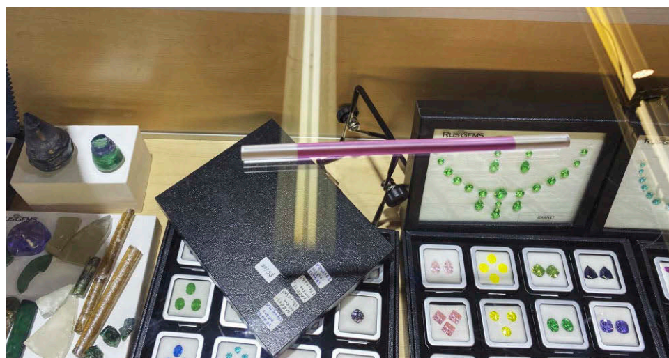
Figure 52. Synthetic ruby rod grown by the flame-fusion technique showing chromium-free ends. Photo by Jennifer Stone-Sundberg; courtesy of RusGems.
