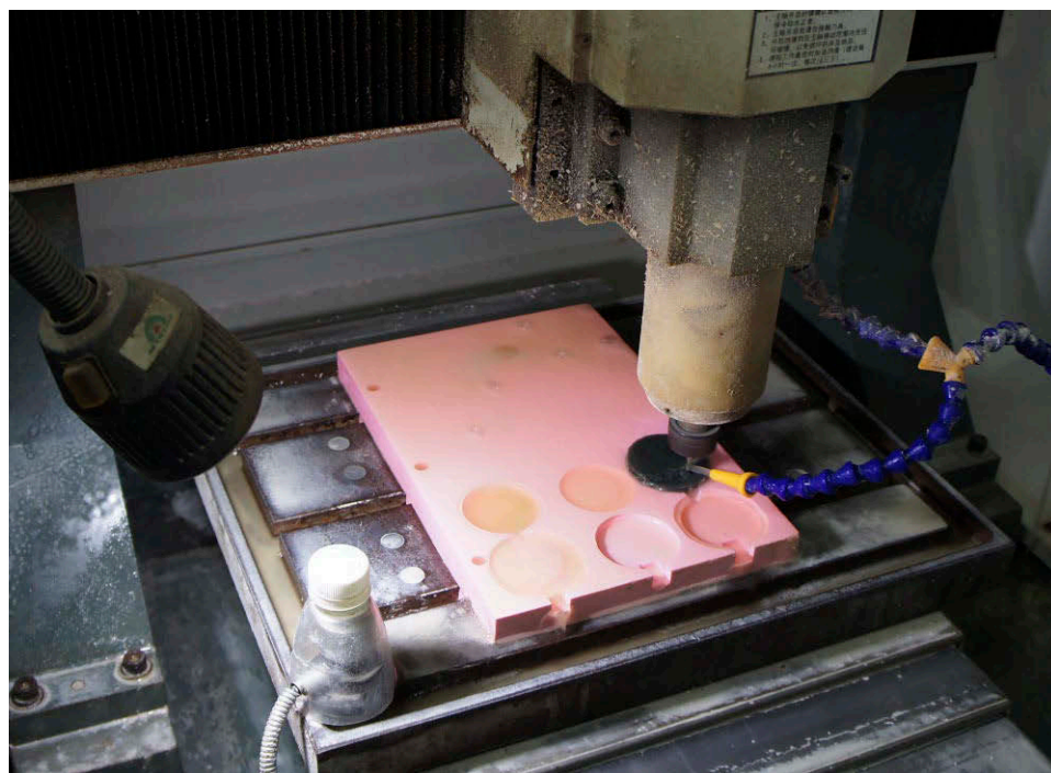
Figure 23. A three-shaft CNC machine engraving tabular nephrite. The machining process is monitored by the computer program. Because the cutting speed is extremely high, the machine needs fluid to keep cool. Photo by Mingying Wang.
