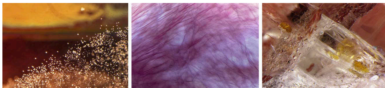
Figure 58. Left: Clouds of copper platelets were observed in numerous Ethiopian sunstones. Field of view 3.13 mm. Center: Dense networks of reddish wispy dislocations were seen in some Ethiopian sunstones, along with a slightly greenish blue bodycolor. Field of view 2.72 mm. Right: Yellowish crystals of what are likely fayalite were seen in one Ethiopian feldspar. These inclusions have also been documented in Oregon sunstone. Field of view 2.82 mm. Photomicrographs by Nathan Renfro.
