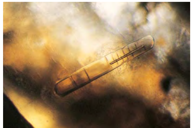
Figure 11. This crystal of clinzoisite in sapphire from Dry Cottonwood Creek displays perfect cleavage; it also hosts a smaller unidentified rod-shaped inclusion. Photomicrograph by John I. Koivula; magnified 35 \times .
