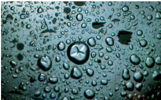
Figure 19. After burning, droplets of charred polymer residue can be seen on the surface of this impregnated synthetic opal; a network of cracks is also visible. Photomicrograph by John I. Koivula; magnified 20 \times .
