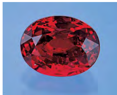
Figure 10. This 1.11 ct spinel from Myanmar appears evenly colored face up, but it is actually strongly color zoned and shows two different refractive index readings.
