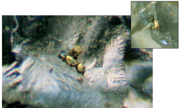
Figure 12. A cluster of gold micronuggets is visible in a surface depression on this sapphire from Dry Cottonwood Creek. Photomicrograph by John I. Koivula; magnified 15 \times . The inset shows a small particle of gold that appears to have been smeared into the surface of the sapphire. Photomicrograph by John I. Koivula; magnified 40 \times .
