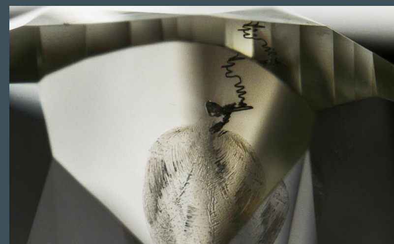
Internal laser drilling is a technique used to open a cleavage crack near dark inclusions to allow bleaching solutions to enter. Instead of a typical drill hole, this treatment is characterized by irregular, wormhole-like channels. Field of view 1.91 mm.
