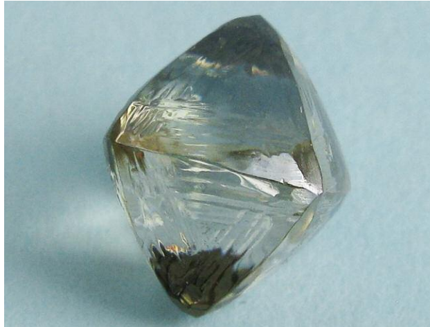
Figure 25. This 5.35 ct sample, submitted as a rough diamond, was identified as synthetic moissanite coated with a diamond film. Photo by V. Pakhomova.
