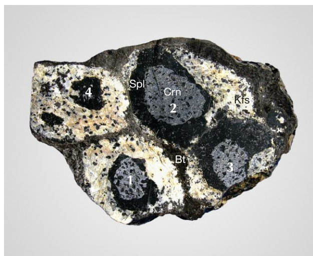
Figure 17. Observed stages of spinel corona formation around corundum grains. As can be seen, from stage 1 to stage 4 the spinel rim around the corundum crystal became progressively thicker, while the corundum core became thinner (until exhausted) and less perfectly hexagonal. Photo by N.N. Khoi.
