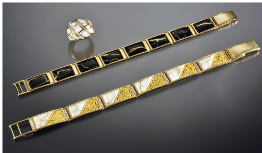
Figure 5. Manufactured gold-in-quartz, set in two bracelets and a ring that were submitted for identification reports.
