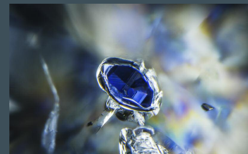
This bright blue kyanite crystal is a rare sight in a faceted diamond. The presence of kyanite suggests that this diamond is from an eclogitic environment. Field of view 2.18 mm.
