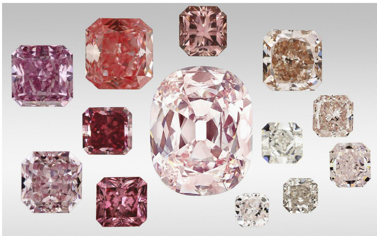
Figure 1. The 34.65 ct Princie (center, photo courtesy of Christie's) is a famous example of a pink diamond colored by NV^{0-} centers. It is flanked by an array of natural brown, brown-pink, orangy pink, purple-pink, and pink diamonds with the far more common cause of color—the 550 nm absorption band. These examples span the diverse color range of pinks submitted to GIA. The photos in this compilation are not imaged to scale.
