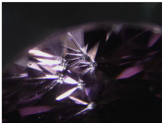
Figure 24. Doubling of the edges, observed near the crown in this synthetic moissanite. Photomicrograph by Aurélien Delaunay; field of view approximately 3.4 mm.
