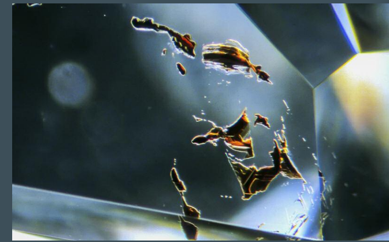
Sometimes thought to be "carbon spots," these chromite crystals reveal their identity by showing orangy brown coloration on thin edges. Field of view 2.10 mm.
